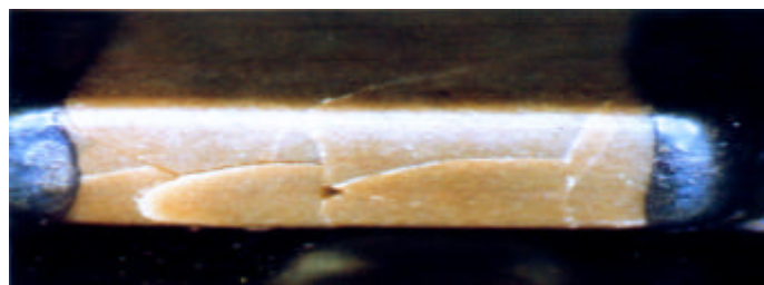
Figure 4. Cracked chip capacitor
