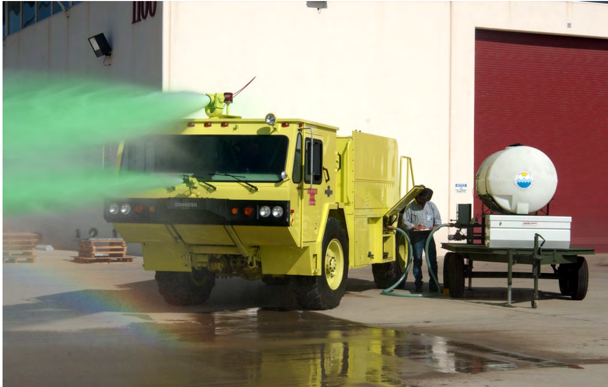
Figure 1. P19 NoFoam System Roof and Bumper Discharge.
