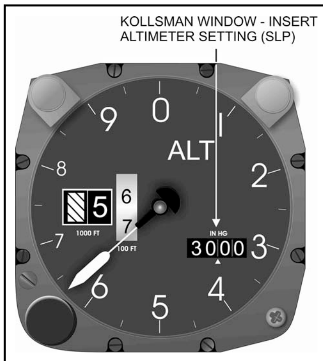
Figure 1-7 Barometric Altimeter (aka Pressure Altimeter)
