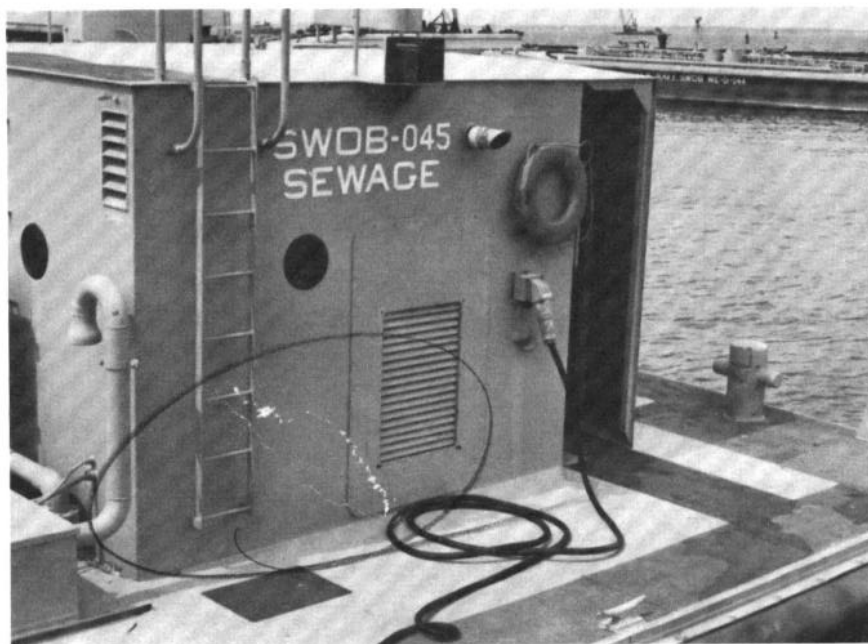
FIGURE 2-8 Shore Power Receptacle
