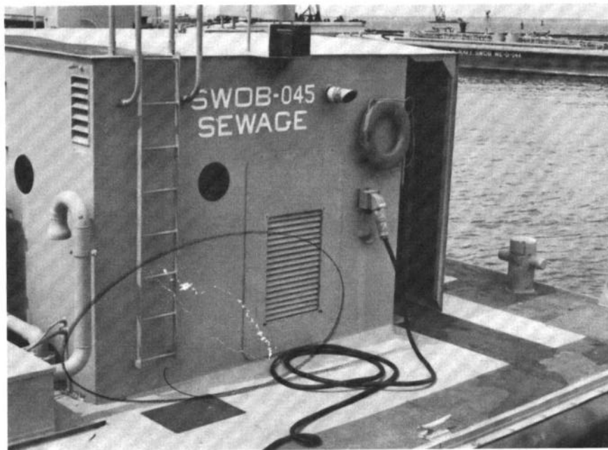
FIGURE 2-8 Shore Power Receptacle
