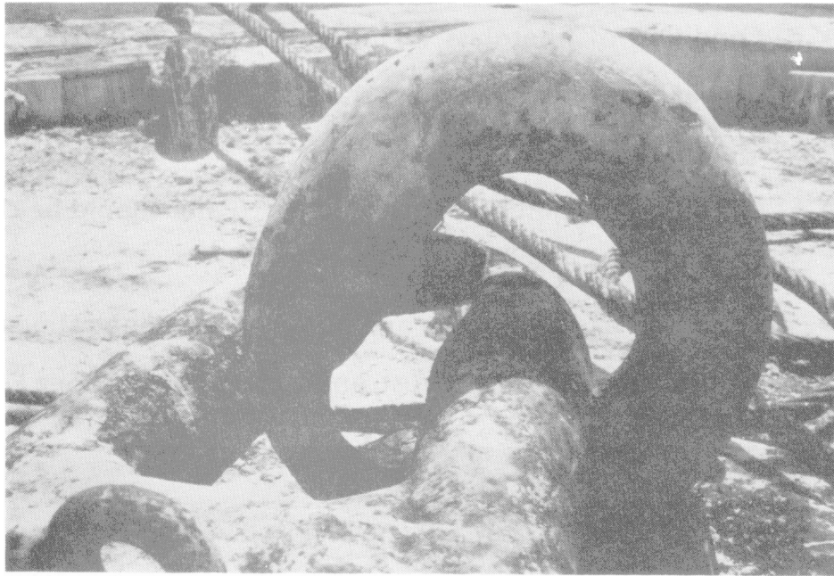
Figure 3-1. An Example of Severely Worn Top Jewelry
