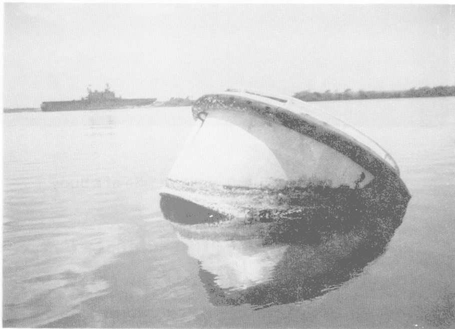
Figure 3-2. Severe Buoy List
