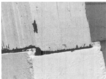
Figure 4-4. (B) Dark area is evidence of localized decay at the top of the metal collar.
