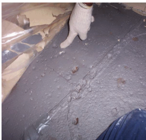
Deeply pitted tank bottom shell plate
