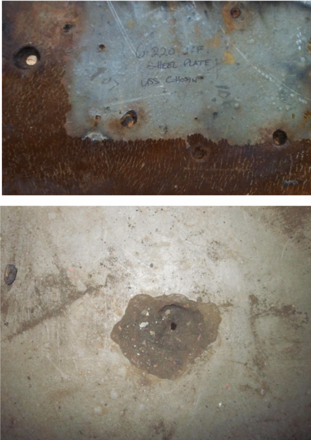
Figure 4-18 Examples of MIC-Produced Isolated Pitting in a Waste Oil Tank
