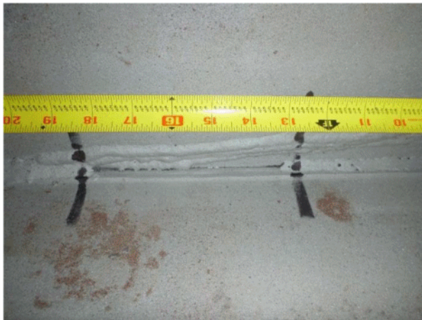
Incomplete Fillet Weld
