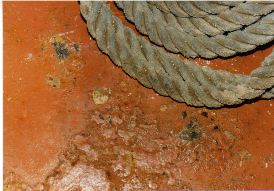
Figure 4-14 Blister-Like Coating Failure Over Rust
