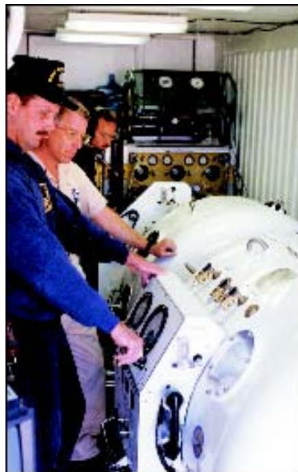
Figure 6-17. Master Diver Supervising Recompression Treatment.
