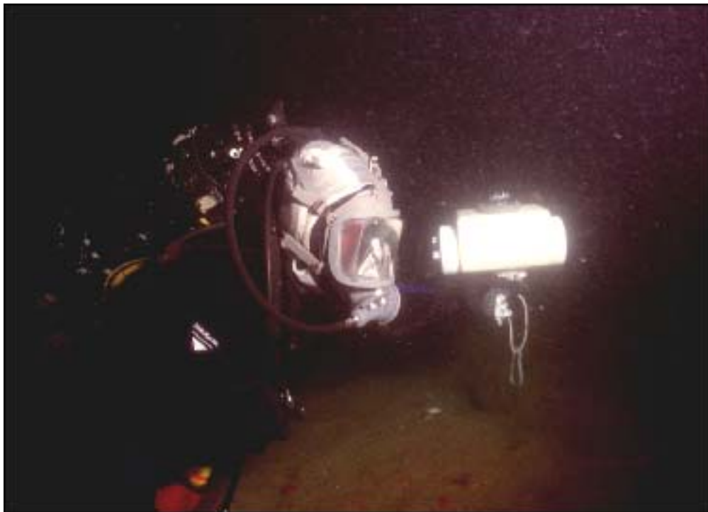
Figure 6-3. Explosive Ordnance Disposal Diving. An EOD diver using handheld sonar to locate objects underwater.
