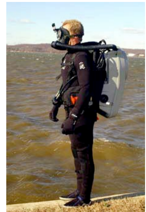
Figure 18-1. MK 16 MOD 1 Closed-Circuit Mixed-Gas UBA.
