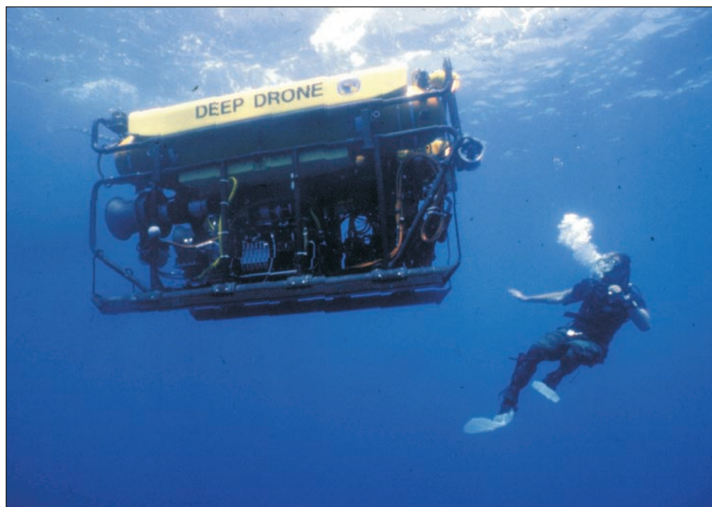
Figure 13-2. Remotely Operated Vehicle (ROV) Deep Drone.
