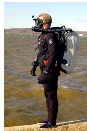
Figure 18-1. MK 16 MOD 1 Closed-Circuit Mixed-Gas UBA.
