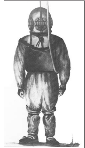
Figure 1-5. Siebe's First Enclosed Diving Dress and Helmet.
