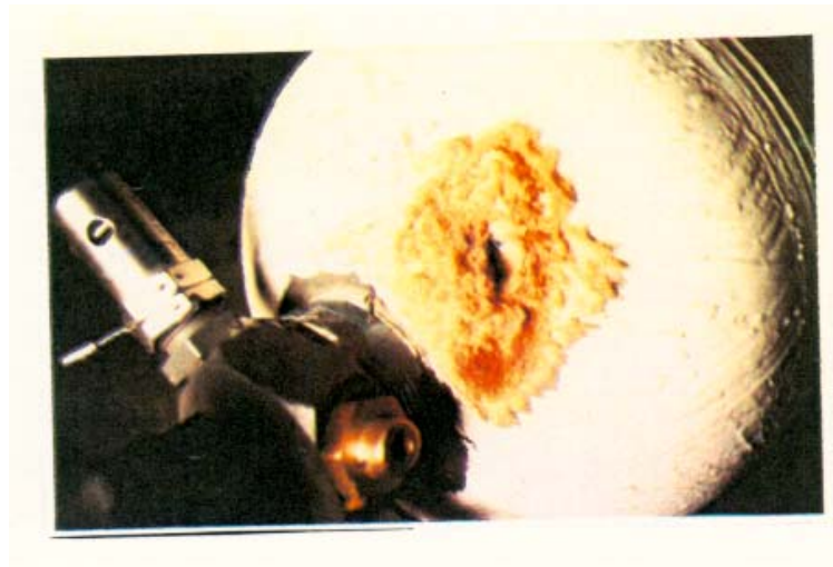
LEVEL 3 STRUCTURAL DAMAGE (CONDEMNED)
