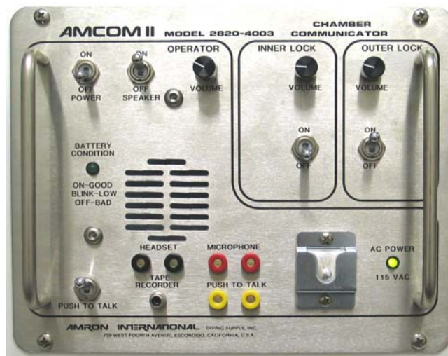
Figure 2-9. Control Console Communications Panel
