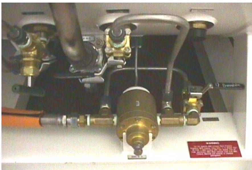
Figure 3-20. BIBS Exhaust Back Pressure Regulator
