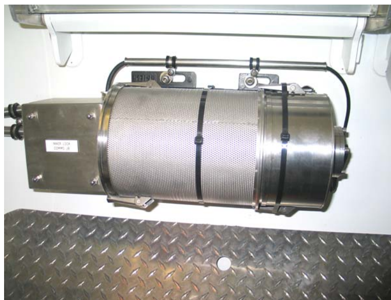
Figure 3-21. Carbon Dioxide (CO 2 ) Scrubber Assembly
