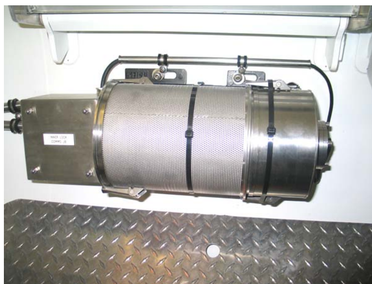
Figure 3-21. Carbon Dioxide (CO 2 ) Scrubber Assembly
