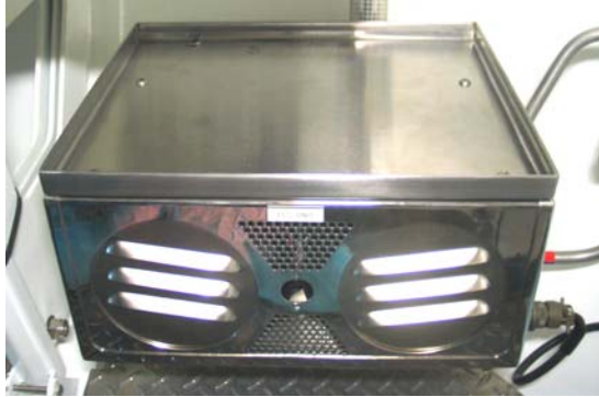
Figure 2-15. Environmental Control System (ECS) Heat Exchanger
