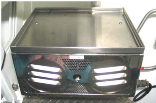
Figure 2-15. Environmental Control System (ECS) Heat Exchanger
