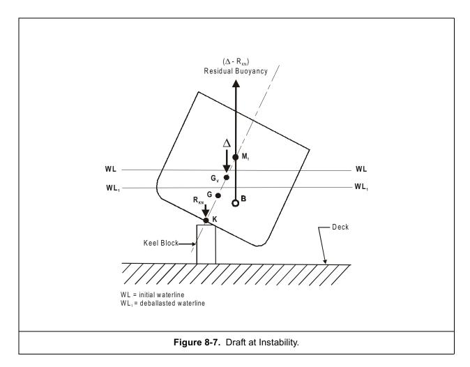
orientation should arrive in a similar condition of list (no more than 0.25 degrees), trim (no more than 1 foot) and draft. It may not be possible to meet these limits with damaged assets.
