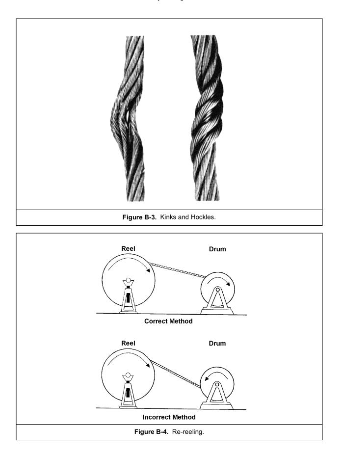
as it is being installed. A reverse bend can make a rope less stable and, consequently, more difficult to handle.
