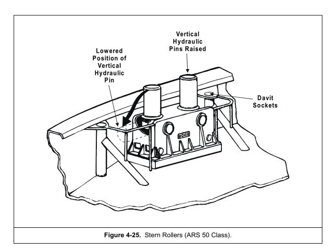
plied at mid-roller height. The towline is usually restrained in a stern roller assembly only under light sea conditions. The vertical stern rollers should always be dropped when maneuvering in restricted waters or rough seas.
