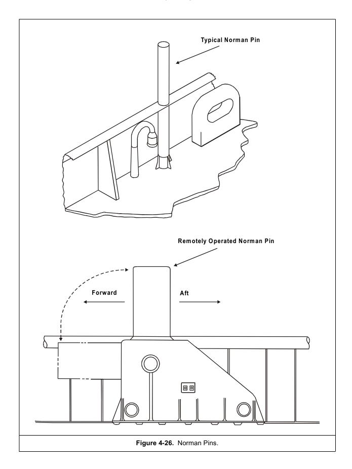
with remote control, the procedures are now safer. Newer tugs and salvage ships, such as the ARS 50 class, have remote controlled, hydraulically operated Norman pins in fixed locations. On board the ARS 50 class, the Norman pins are set to drop when the lateral force at mid-barrel height exceeds 50,000 pounds. The hazard potential is formidable. When the pins start inclining toward the horizontal, the wire (with 25 tons force propelling it) can jump the pin and sweep forward.
