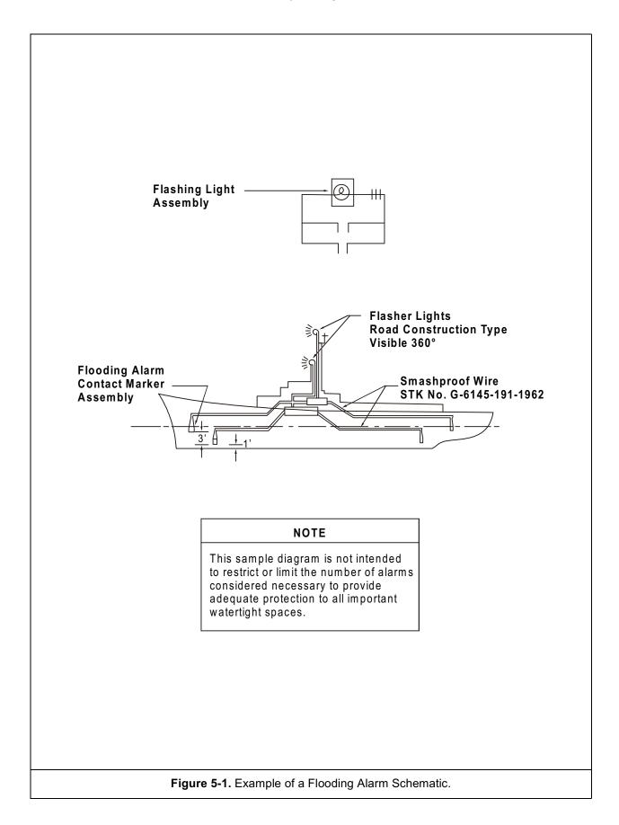
provide coverage of major hull subdivisions. Alarms should be securely rigged and properly serviced to ensure performance and reliability.
