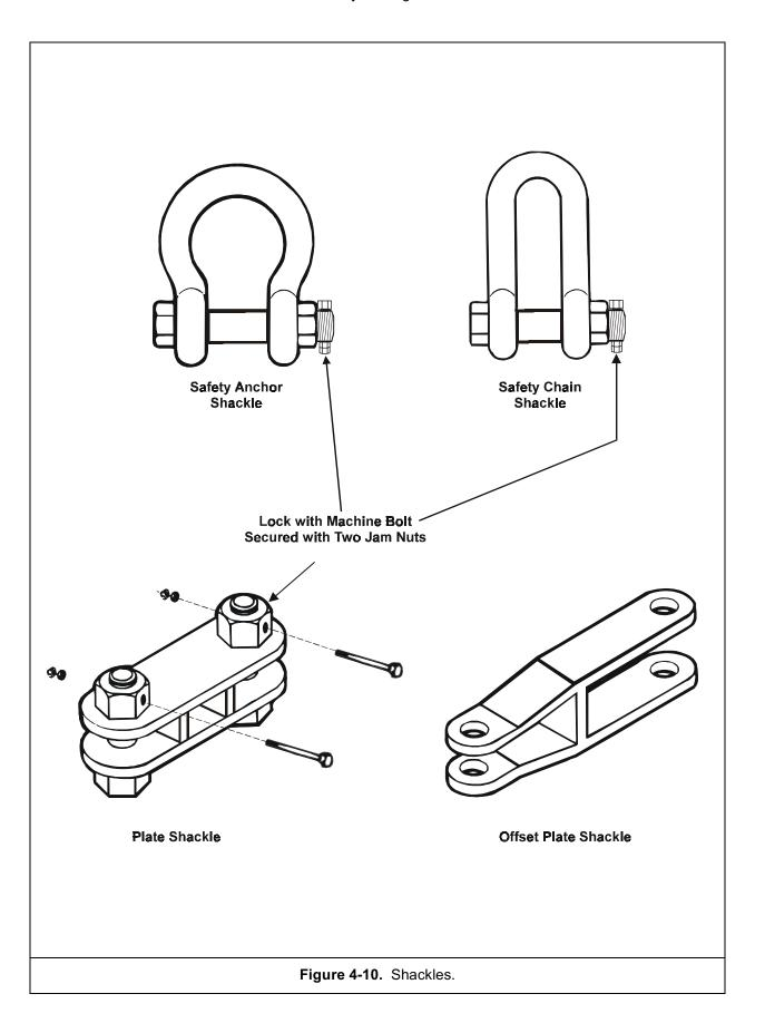
tion are anticipated during the tow it is good practice to procure additional properly sized locking bolts prior to getting underway. Cotter keys should not be used in towing.
