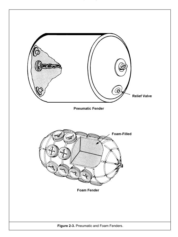
get out of step, the fender can be rolled upward between the two ships and pop out onto the deck of the one with the lower freeboard.
