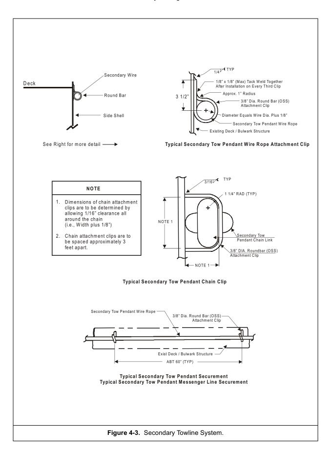
For an emergency tow, a makeshift connection, such as a heavy chain wrapped around a strong foundation, may be used. In every case, the material condition of the fittings and structures should be carefully inspected.
