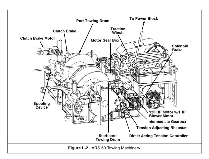
When the clutch is released, the winch can be overhauled by the hawser to provide for free release of the hawser in an emergency. Some traction winches have an automatic tension payout capability, but automatic reclaim is rare on fiber line systems because of the hawser storage system described above.Controls and Instrumentation
