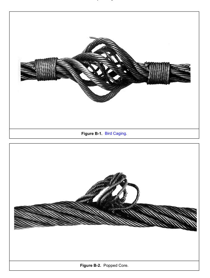
rope when a failure in the towline or its connections allows the rope to rebound from an overload. These conditions also can result from operating a wire rope through an undersized sheave groove (see Figures B-1 and B-2).
