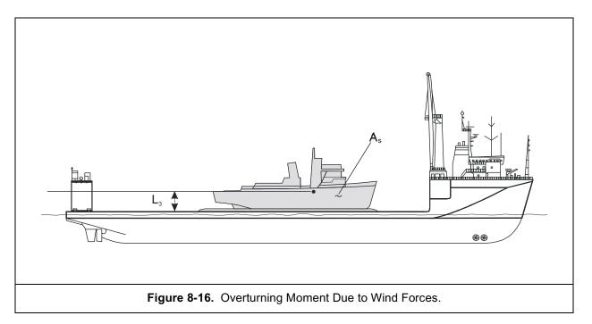
To calculate the overturning moment  $(M_r)$  associated with athwartships motion, the weight of the asset is multiplied by the height of the center of gravity above the asset's keel. This is then multiplied by an acceleration factor similar to that calculated for keel blocks.
