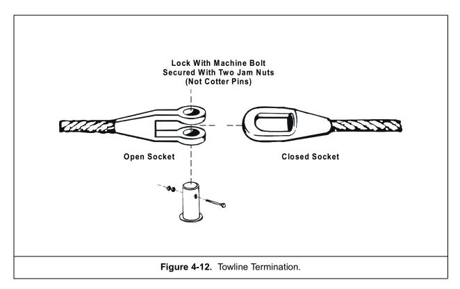
individual wires. This broomed end is inserted into the socket and secured in place with the poured zinc. Epoxy-type poured sockets are not suitable for towing purposes.
