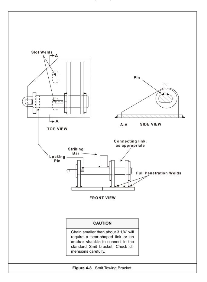
main pin to slide out of the pear-shaped link. The design uses no shackle. This style of towing attachment, like the vertical free-standing padeye, is susceptible to tripping loads and is dependent upon the fairlead chock.
