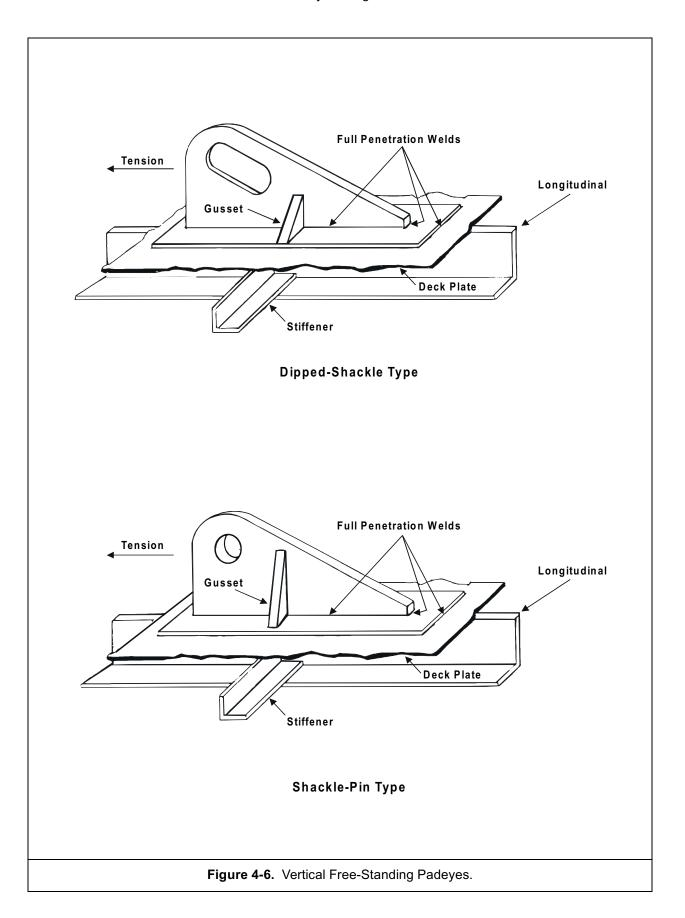
The vertical free-standing padeye may have a higher attachment point than the horizontal padeye. This makes for larger loading moments on the structure itself and on the attachment system to the ship deck or frame structure. This in itself is not a disadvantage if the design is proper and those who rig the system understand it.
