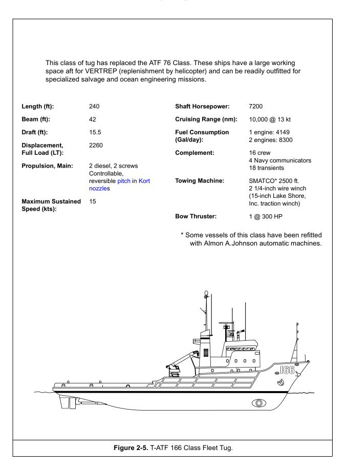
that can handle synthetic hawsers up to 15 inches in circumference. The class was originally equipped with a single-drum, diesel driven, non-automatic SMATCO towing winch relatively common to the offshore oil industry (see Figure L-3). Some members of this class have been refitted with an (Almon A. Johnson) electrohydraulic automatic towing machine (see Figure L-4).
