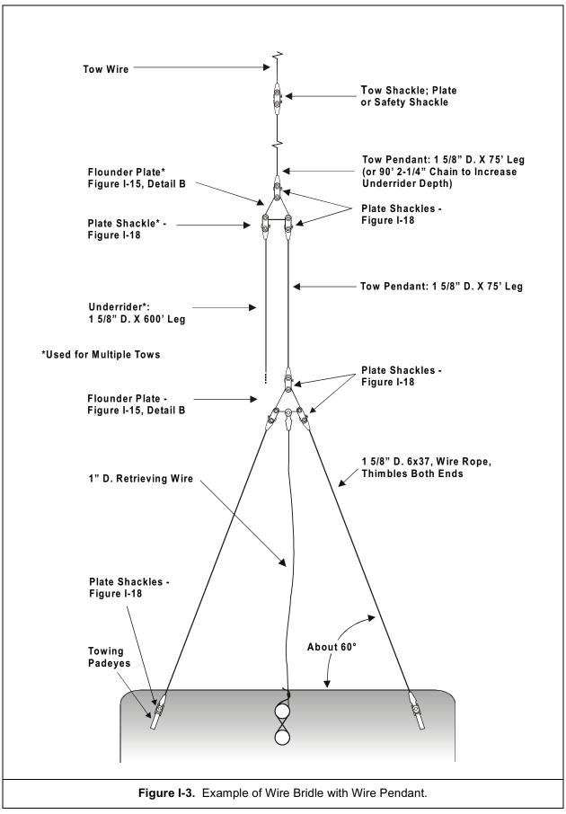
flounder plate with the two bridle legs connected at its base and the apex usually connected to the lead chain and/or towing pendant, which in turn is connected to the tow hawser.
