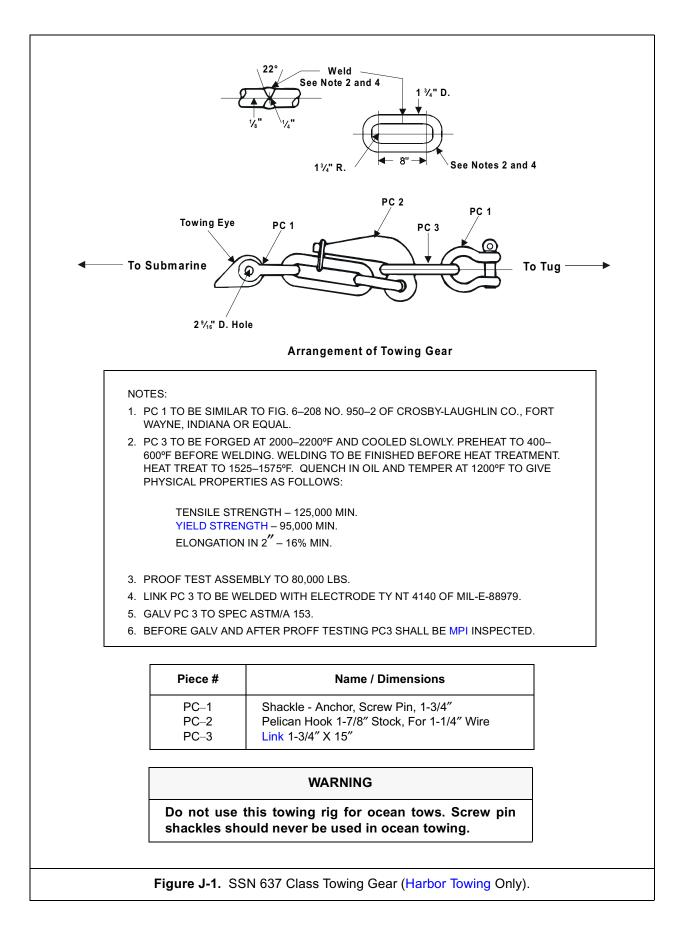
the submarines towing plans are  $1^{3}/4$ -inch screw-pin anchor shackles. Do not use these shackles for towing. Use only comparable safety shackles. Note that the standard tow pad will accept the pin of a standard 2-inch safety shackle. The tug should provide more robust gear if time permits.
