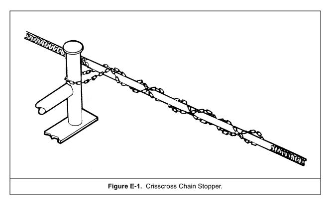
In a situation where a carpenter stopper is not readily available, the hawser can be stopped off with a chain. If using a chain stopper, be very careful not to damage the hawser (see Figure E-1).
