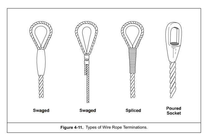
junction with suitable dies. The swaged fittings are usually made of special alloy steels. An advantage of this process is low cost and high efficiency.
