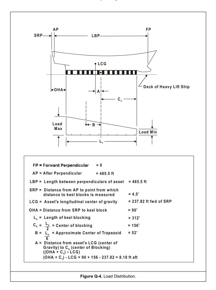
pected local stress on the keel blocks, and the load carrying capacity of the cargo deck of the heavy lift ship. The equation for LoadMax returns a value in tons per foot.
