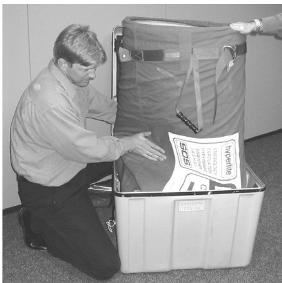
Figure 4-3. Folding The Flexible Tube – Third Fold
