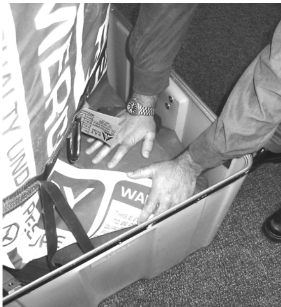
Figure 4-2. Folding The Flexible Tube – Second Fold
