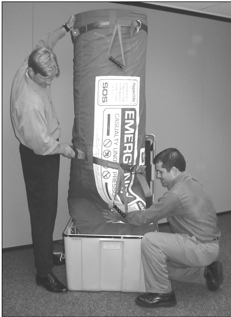
Figure 4-1. Folding The Flexible Tube – Primary Fold
