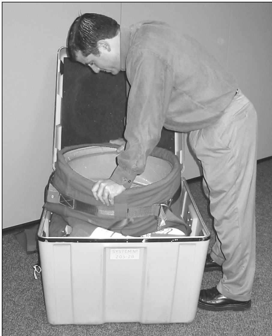
Figure 4-4. Folding The Flexible Tube – Fourth Fold
