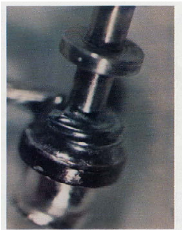
Figure 2-3. Turret Post Connections
