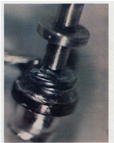
Figure 2-3. Turret Post Connections
