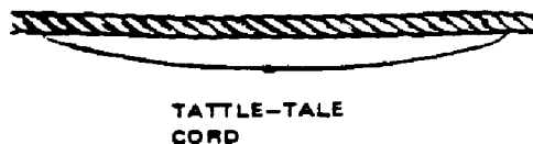
Figure 613-2-28. Relaxed Synthetic Fiber Rope
