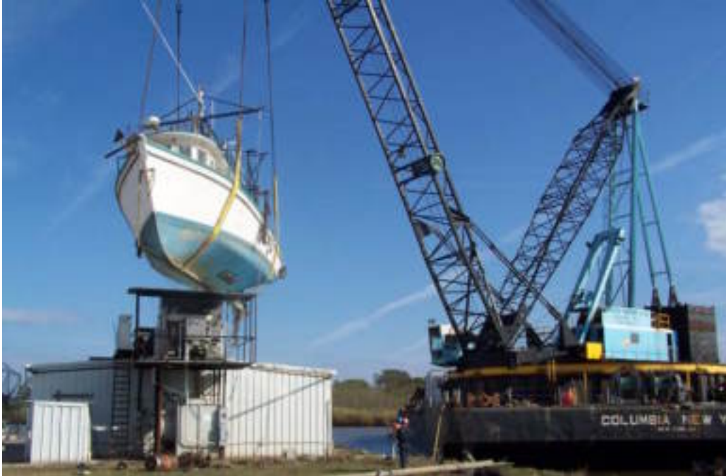
Figure 5-16. Donjon's derrick barge Columbia NY repositions the wooden shrimp vessel Michele Rose from its stranded position ashore to the waterway in Intracoastal City, LA.
