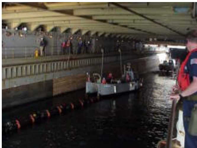
Skimmers in welldeck - LSD ballasted down aft
