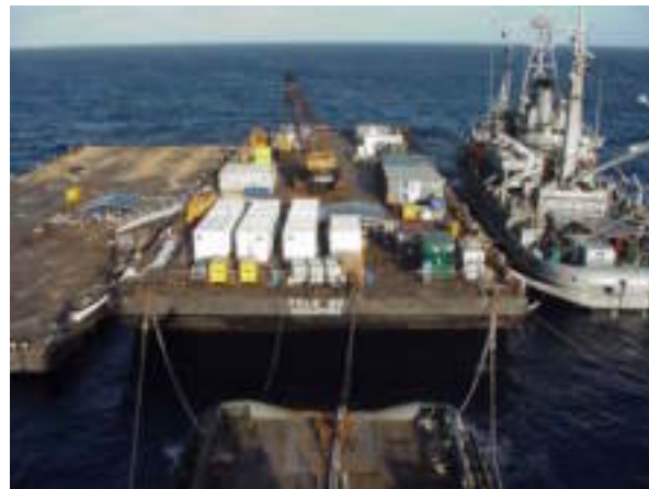
FELS-20 as a work platform in a 6-point moor
