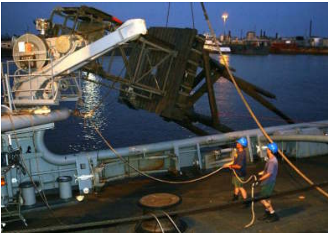
Figure 5-20. USS GRAPPLE lifting a channel marker clear of the channel in Mobile, AL.
