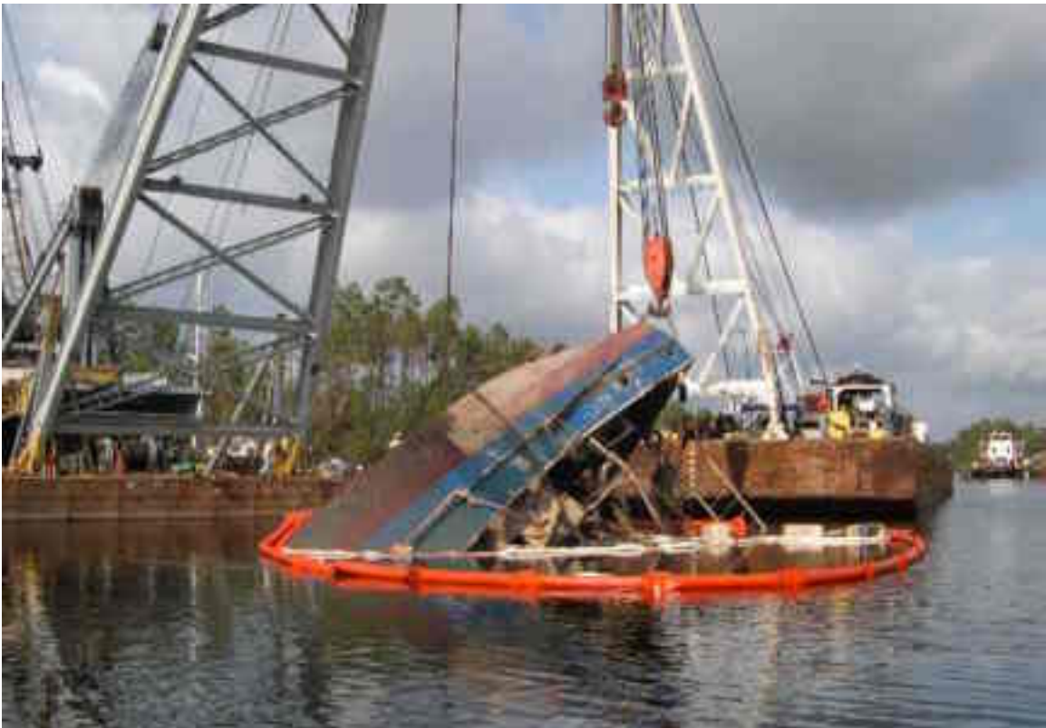
Figure 5-18. Fishing boat being raised out of the Harris County Industrial Canal by MDSU TWO and SUPSALV-leased derrick barges.
