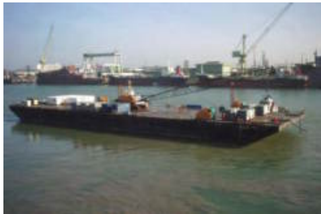
Deck Barge FELS-20 specially configured as a work barge
