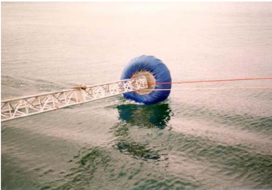
VOSS Outrigger Assembly OA0010 (Deployed)
