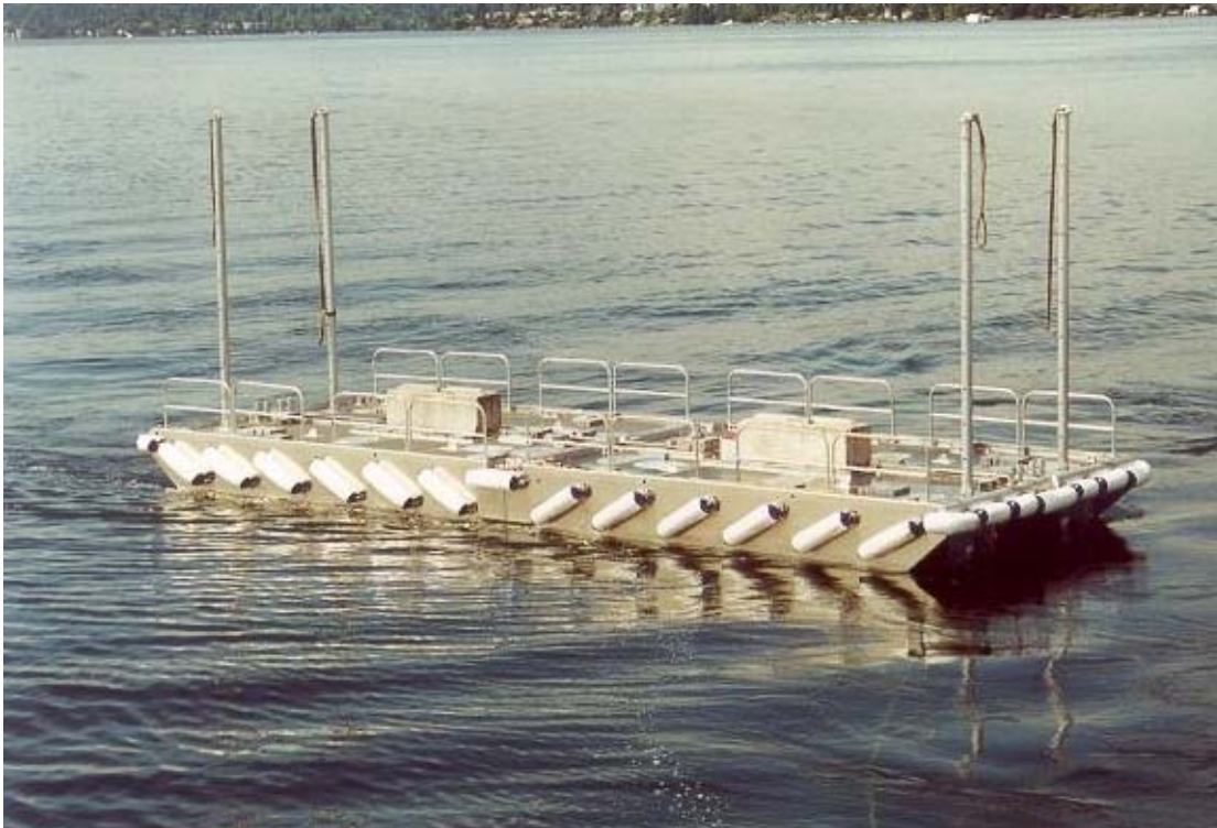
Supersectional Barge Assembly (two single sectional assemblies)
