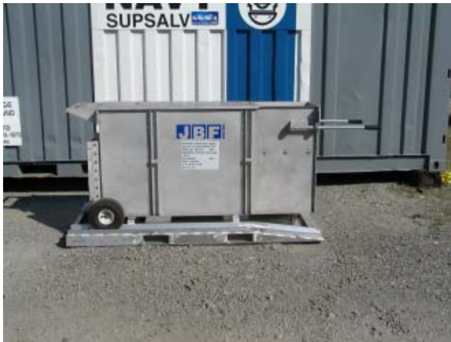
Moving Inclined Belt Skimmer SK0030
