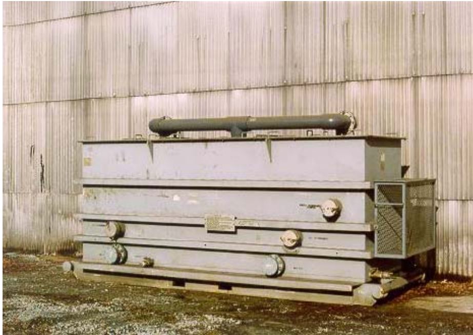
100-Gpm Gravity Plate Oil/Water Separator SR0815
