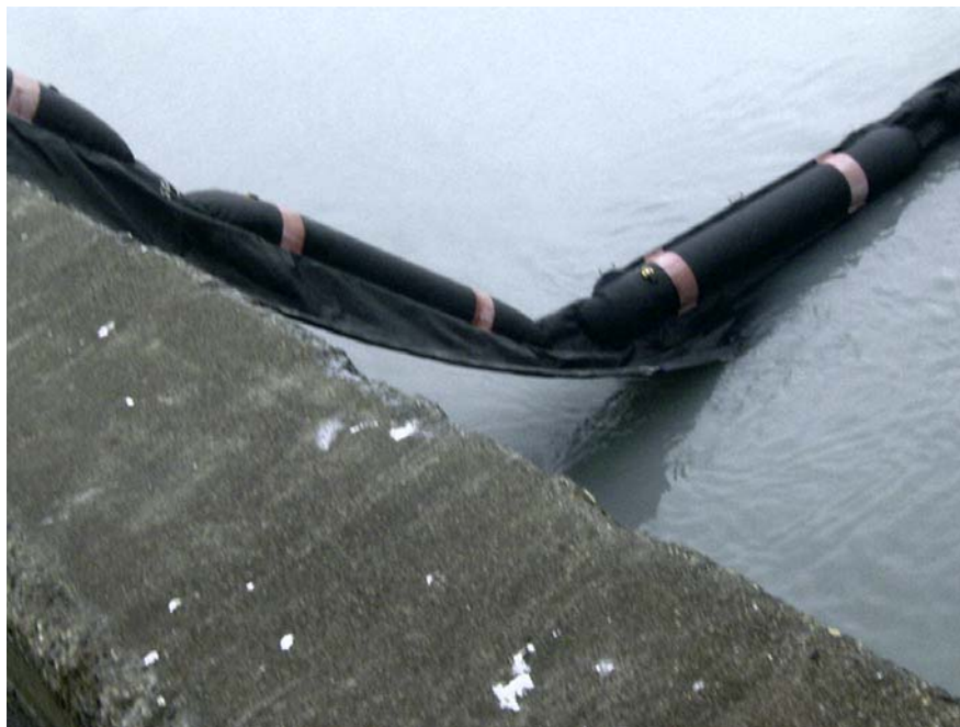
42" x 55' Oil Containment Boom, Model USS-42 BM0738
