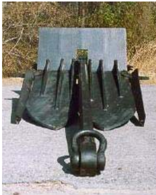
500-Lb Stato Anchor with Short Mud Palm and Folding Stabilizers AN0152
