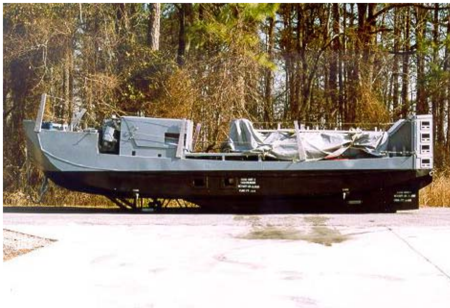
Modified Oil Skimmer SK0711 Without Side Hull
