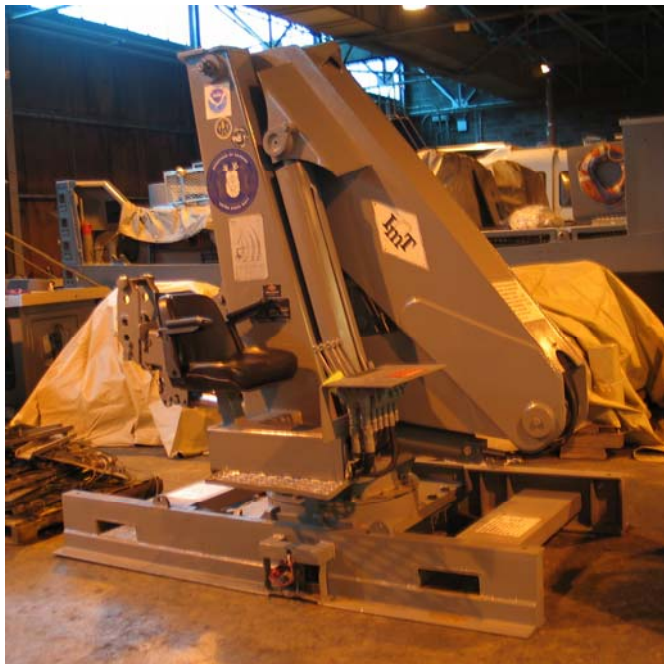
40' Knuckle Boom Portable Hydraulic Crane CR0040
