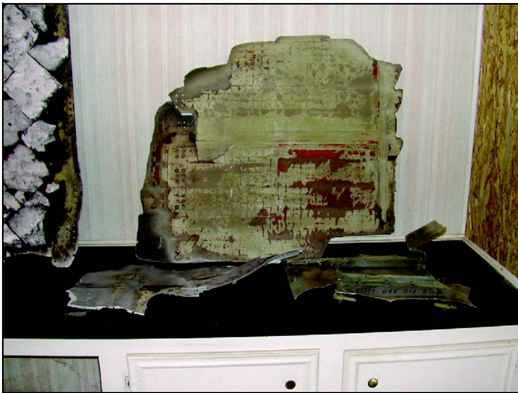
Figure 3-14. Actual Shuttle Pieces Used as Test Targets.
