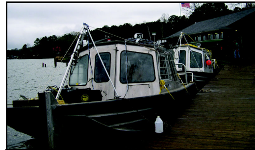
Sector Scan Unit Mounted on its Tripod Staged on Bow of Dive Boat
