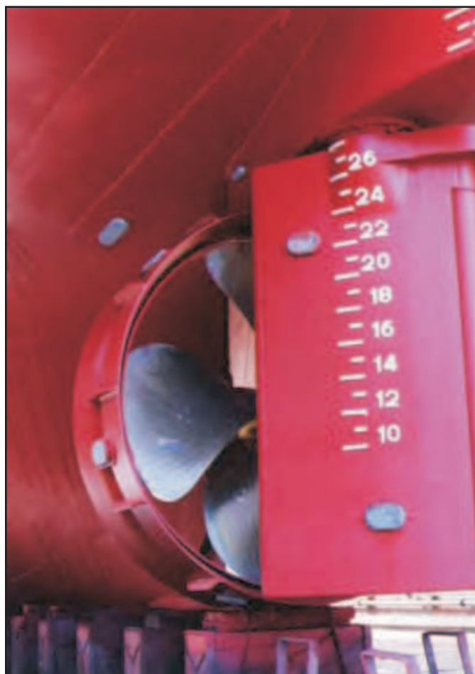
Figure 8-4. Kort Nozzle.
