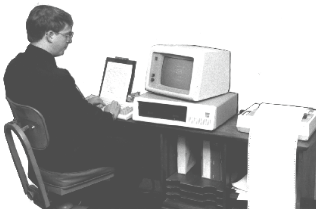
Figure 1-12.—Typical microcomputer system with display, keyboard, floppy disk drives, and printer.
