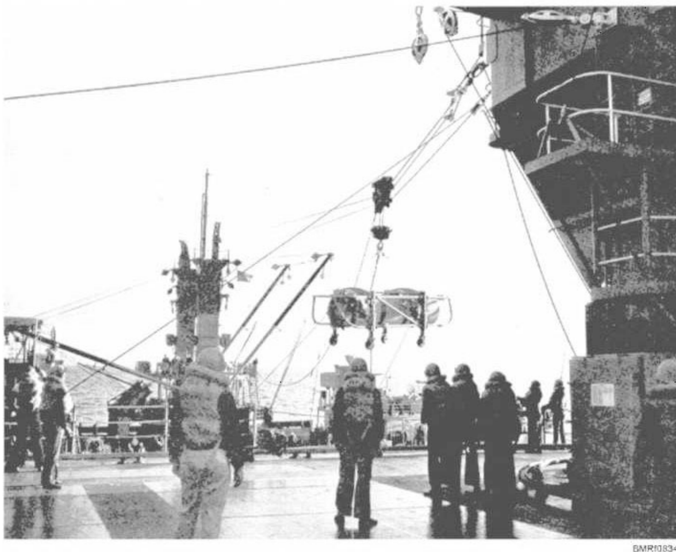
Figure 8-34.—An AE highlines a missile to a guided-missile ship during replenishment at sea.
