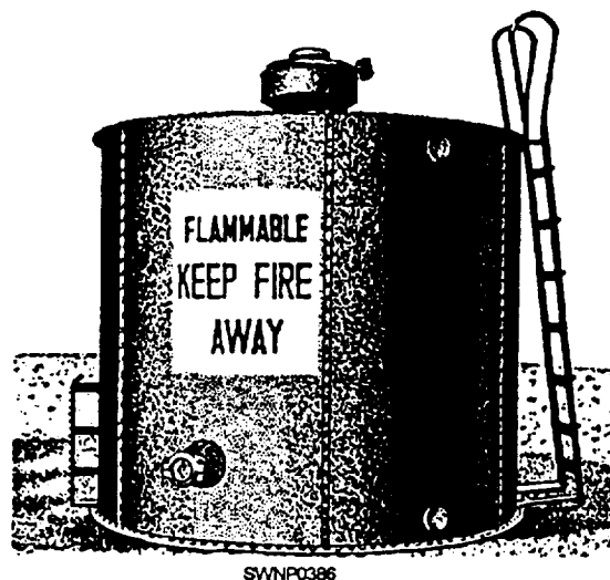
Figure 9-1.—100-barrel capacity, vertical, bolted steel tank.
