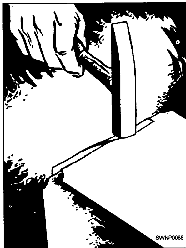
Figure 2-71.—Closing a Pittsburgh lock seam
