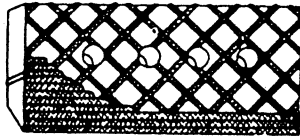
Figure 7-48.—Wearfacing bulldozer end bits.
