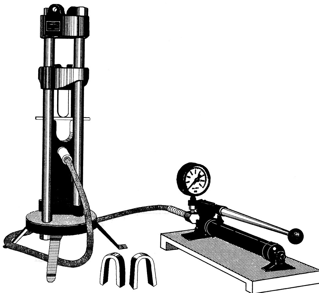
Figure 7-64.—Testing machine for making guided-bend tests.
