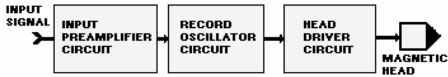
Figure 5-4.—FM record electronics.
