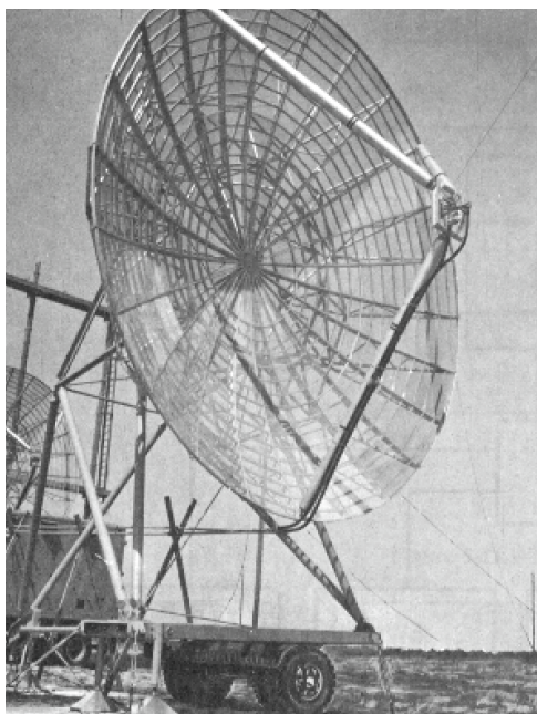
Figure 5-9.—Mobile 30-foot tropospheric-scanner antenna.
