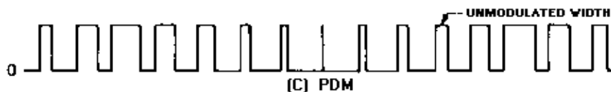
Figure 2-43C.—Pulse-time modulation (ptm). PDM.
