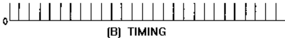
Figure 2-42B.—Pulse-amplitude modulation (pam). TIMING.
