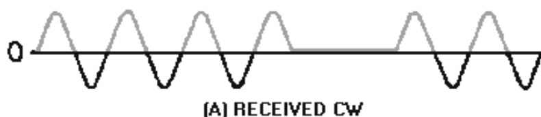
Figure 3-1A.—Cw demodulation. RECEIVED CW.
