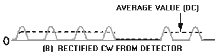
Figure 3-1B.—Cw demodulation. RECTIFIED CW FROM DETECTOR.
