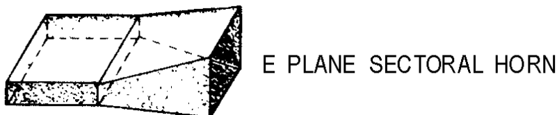
Figure 1-44A.—Waveguide horns. E PLANE SECTORAL HORN.
