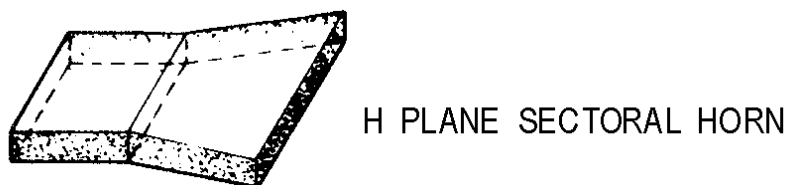
Figure 1-44B.—Waveguide horns. H PLANE SECTORAL HORN.
