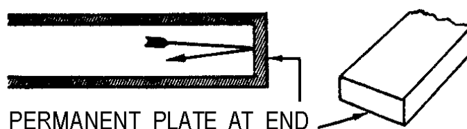
Figure 1-45D.—Terminating waveguides.
