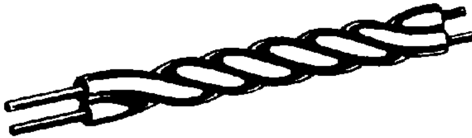
Figure 3-4.—Twisted pair.
