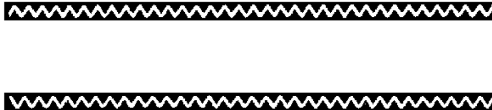
Figure 3-12.—Distributed resistance.
