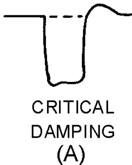
Figure 3-36A.—Waveform damping. CRITICAL DAMPING.
