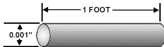
Figure 1-3.—Circular-mil-foot.
