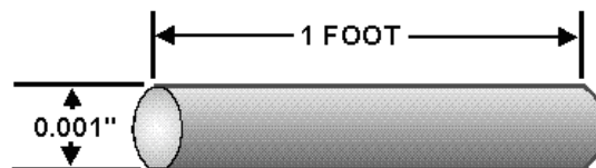
Figure 1-3.—Circular-mil-foot.
