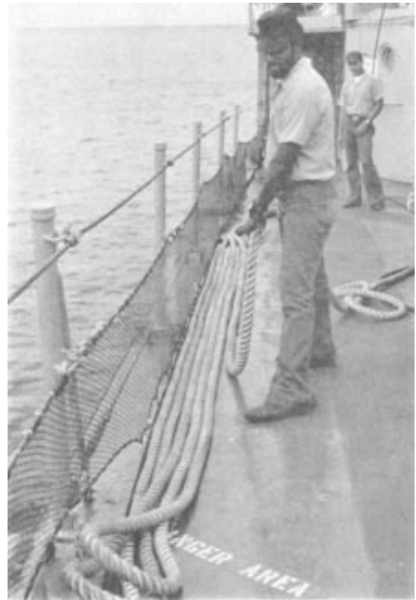
Figure 3-4.—Faking down a line.
