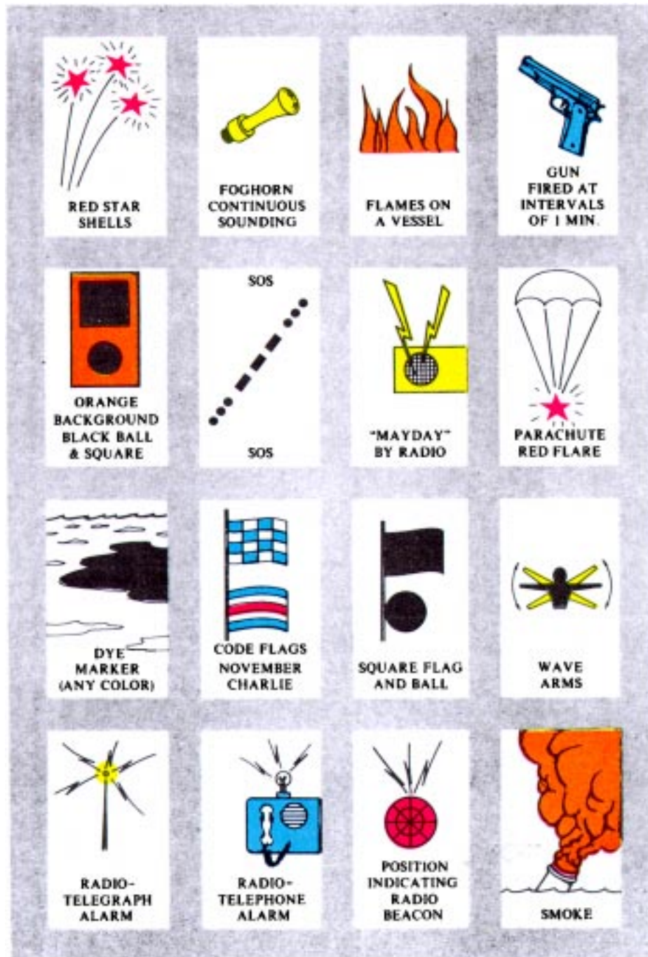
Figure 5-17.—International/inland distress signals.
