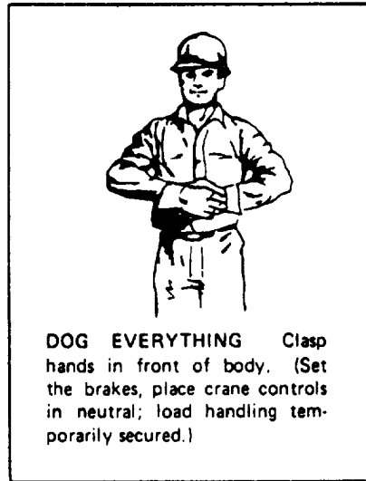
Figure 4-23.—Hand signals used in crane operations, sheet 2.
