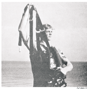
Figure 5-12. Step 1, donning the OBA.
