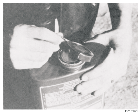
Figure 5-16. Step 5, removing the tear-off cap.
