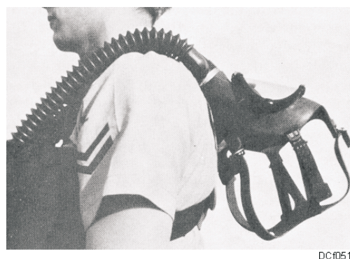
Figure 5-15. Step 4, donning the OBA.
