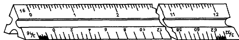
TRIANGULAR SCALE 16, 3/16 AND 3/32 SCALES ARE SHOWN. 16 SCALE IS SUBDIVIDED INTO SIXTEENTHS. ALL OTHERS ARE SUBDIVIDED INTO TWELFTHS.
