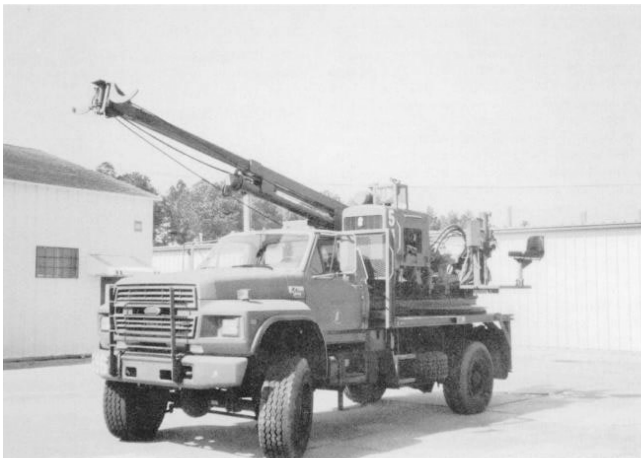
Figure 4-39.—Earth auger.
