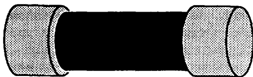
Figure 5-63.—Ferrule type of fuse.
