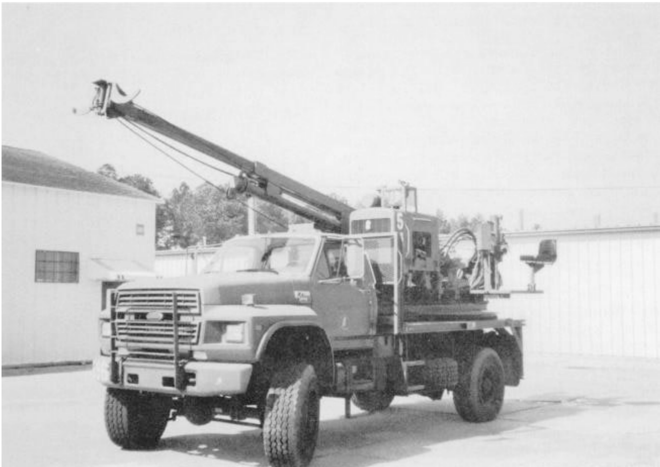
Figure 4-39.—Earth auger.
