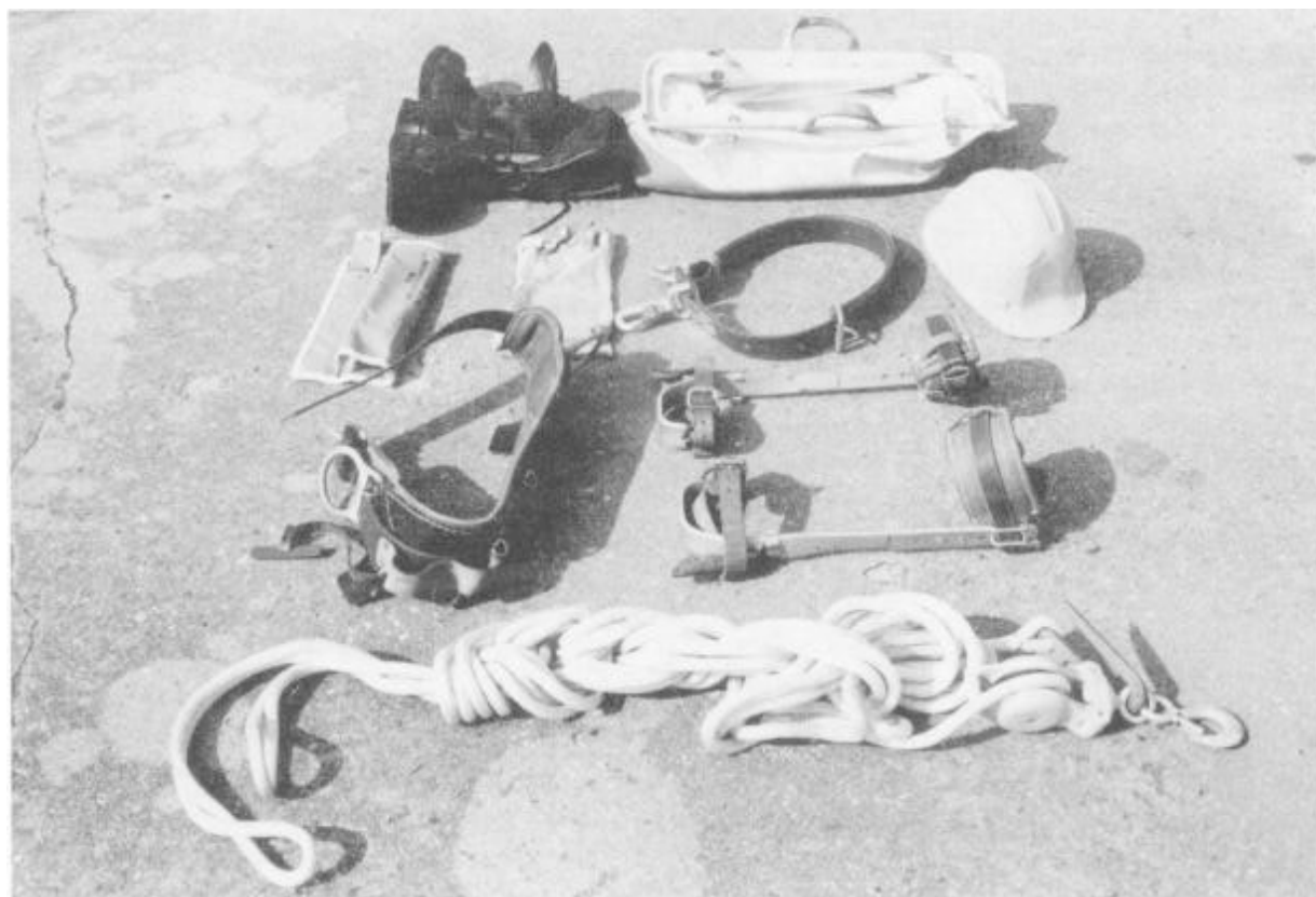
Figure 4-73.—Pole climbing equipment.
