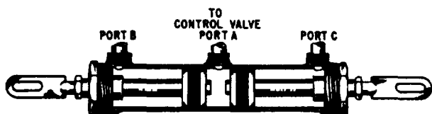
Figure 10-7.—Three-port, double-acting actuating cylinder.
