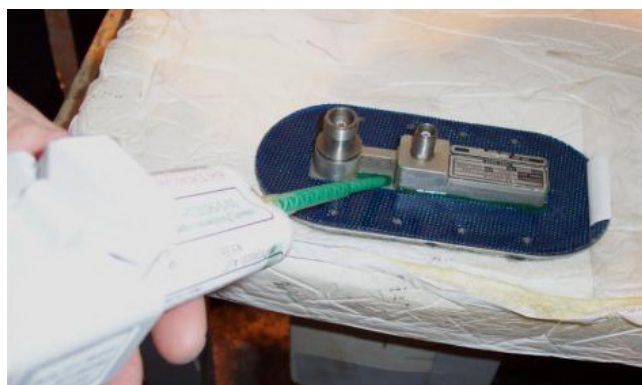
Figure 6-4. Application of Self-Leveling Green Sealant
