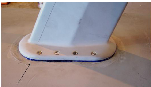
Figure 6-6. Typical Gel Squeeze-Out Around Perimeter of Antenna
