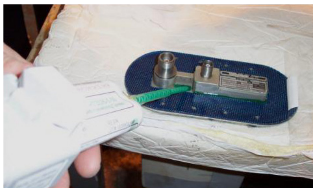
Figure 6-4. Application of Self-Leveling Green Sealant
