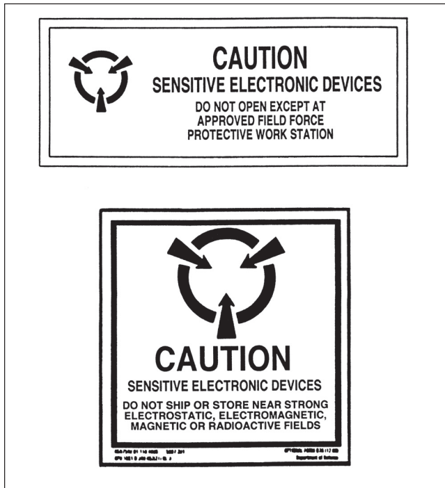
Figure 8-4. Examples of Typical Markings on ESD Sensitive Item Package
