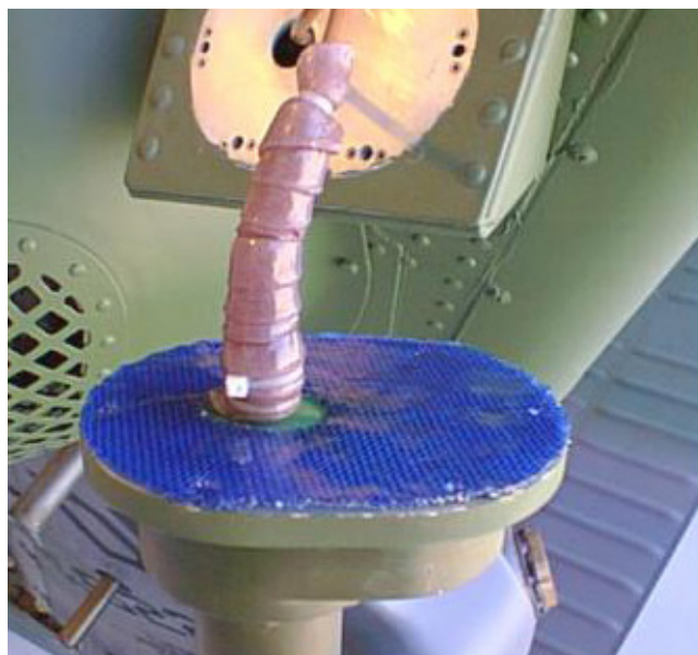
Figure 6-5. Stretch Seal Protective Wrap Applied to Antenna Connector
