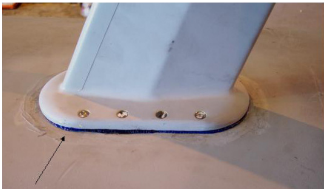
Figure 6-6. Typical Gel Squeeze-Out Around Perimeter of Antenna
