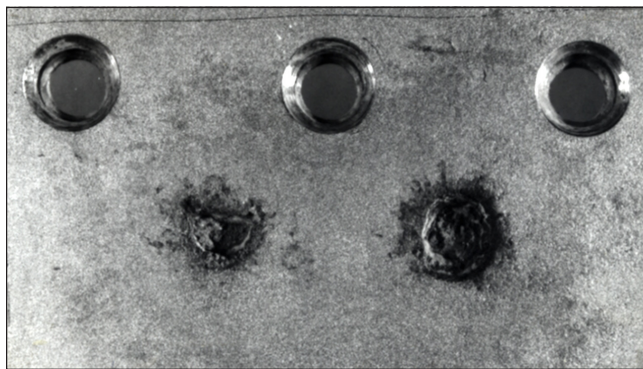
Figure 3-7. Spot Weld Corrosion
