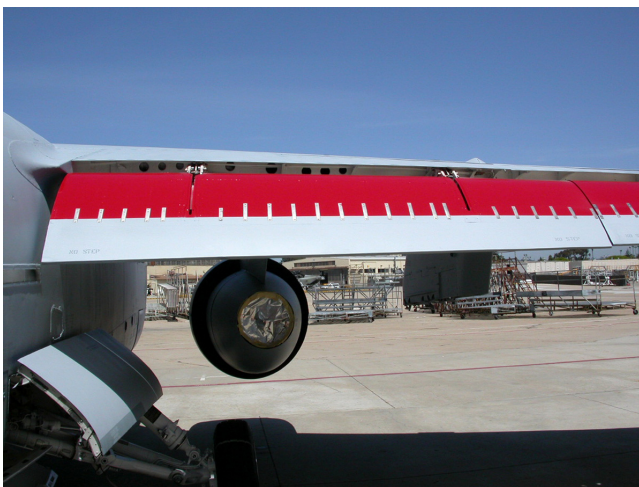
Figure 3-12. Flaps Lowered to Expose Recess Areas
