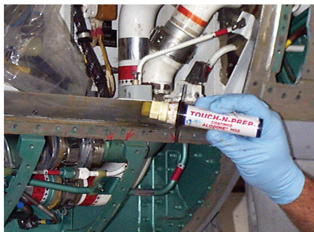
Figure 5-3. Application of TNP Pen on Aluminum Substrate
