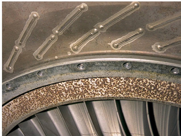
Figure 3-22. Hot Corrosion on Engine Components
