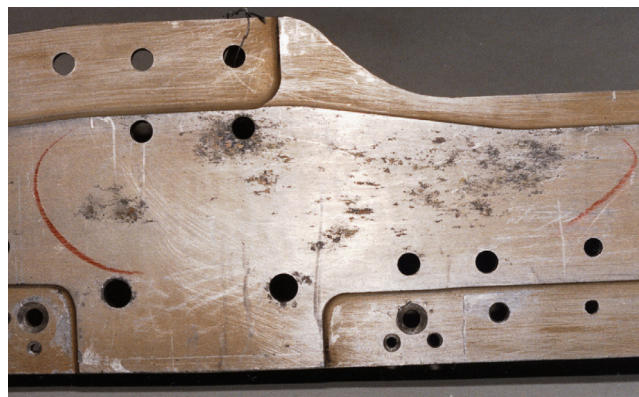
Figure 3-10. Pitting of an Aluminum Wing Assembly
