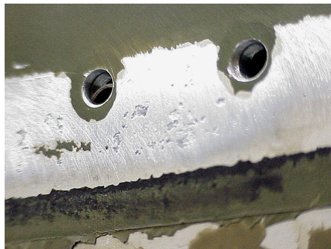
Figure 3-20. Fretting Corrosion
