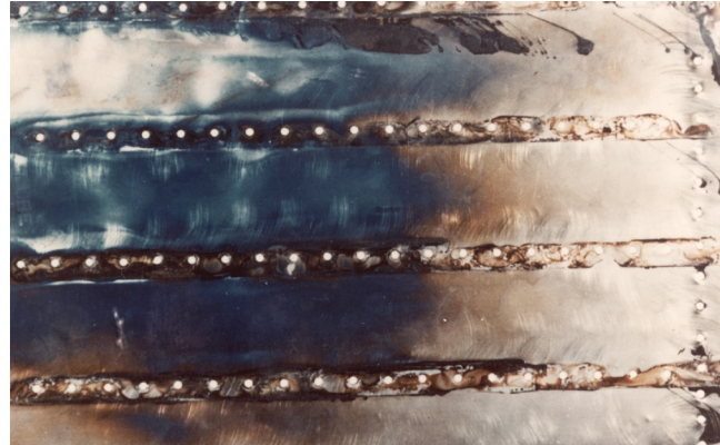
Figure 3-26. Color Changes in Titanium Due to Heating
