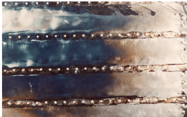
Figure 3-26. Color Changes in Titanium Due to Heating
