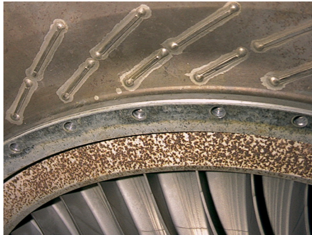
Figure 3-22. Hot Corrosion on Engine Components
