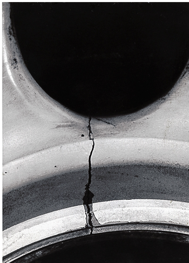
Figure 3-19. Cracking (Typical of Stress Corrosion or Corrosion Fatigue)
