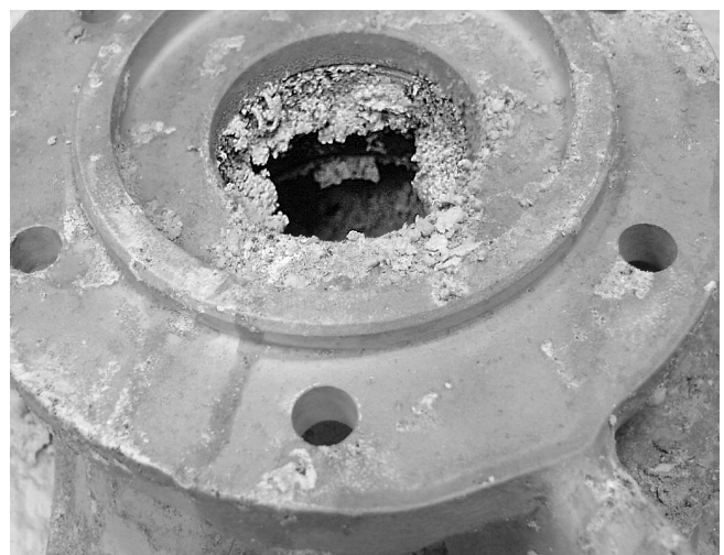
Figure 3-24. Magnesium Corrosion Products
