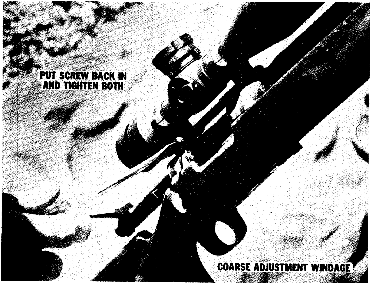
Figure 3-14. Course Adjustment with Scope Base for Zeroing.
