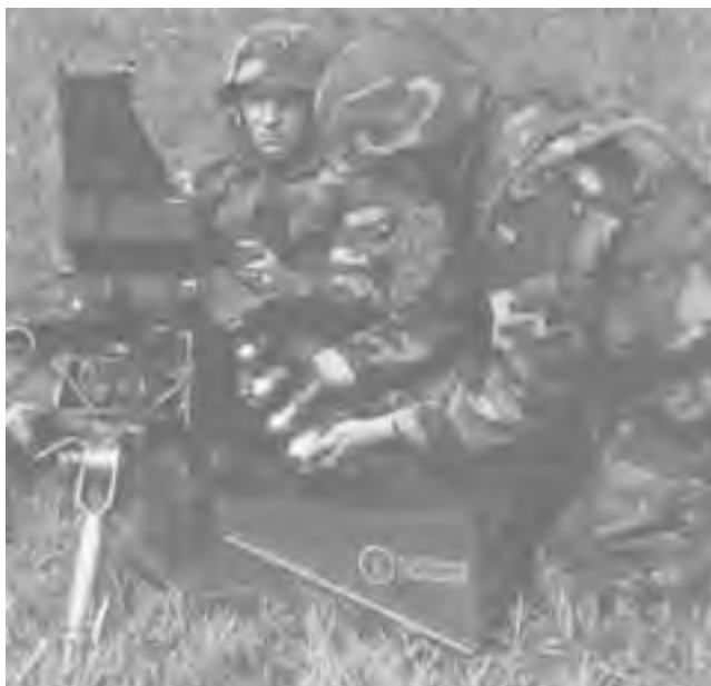
Figure 5-55. Inserting the First Round into the Feeder.
