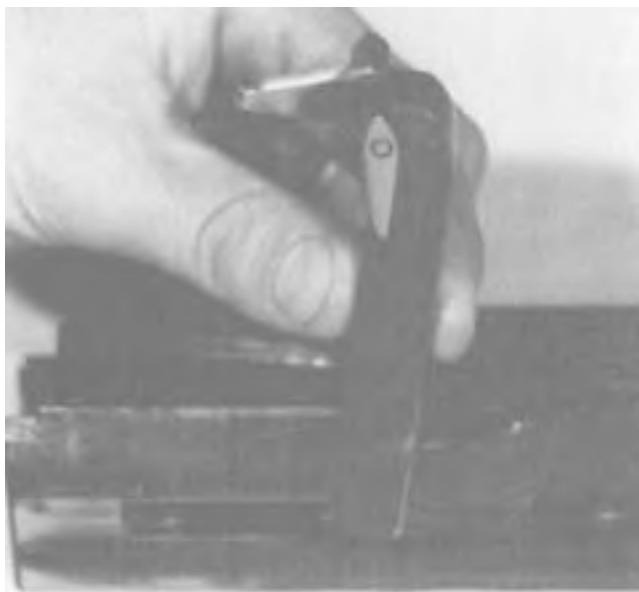
Figure 4-20. Removing the Extractor.
