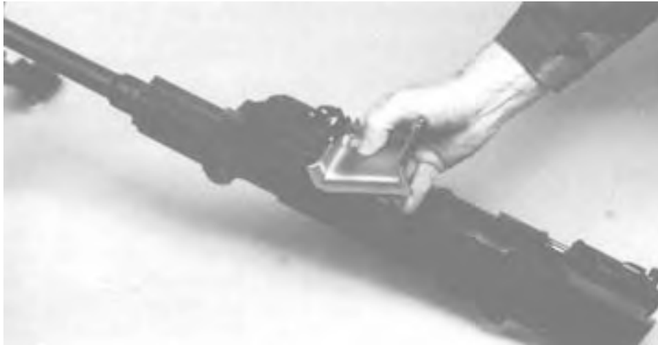
Figure 3-21. Aligning the Feed Tray Guides.
