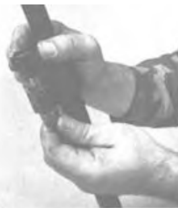
Step 2. Removing Collar From Gas Plug.
