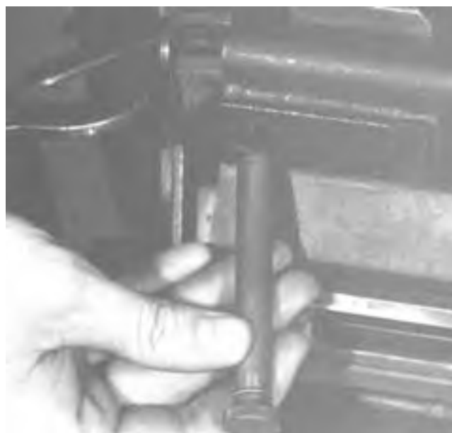
Figure 5-7. Removing the Bolt and Backplate Pin.
