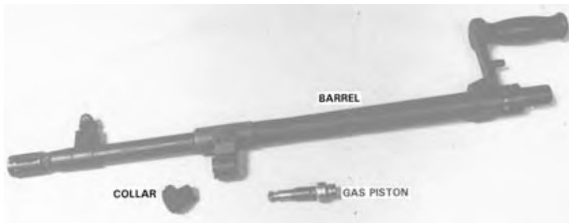
Figure 3-18. Barrel Group, Detailed Disassembly.
