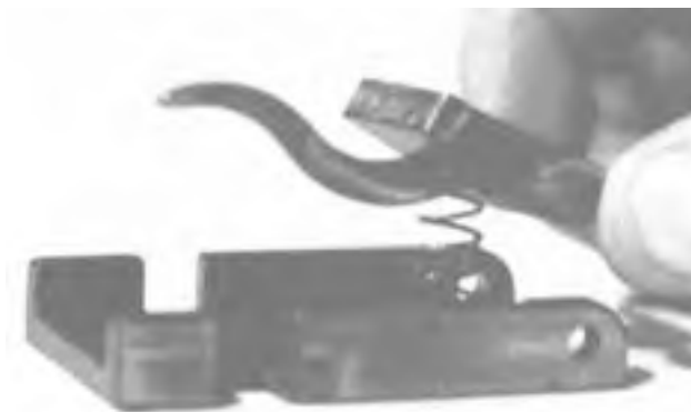
Figure 4-42. Removing the Belt Feed Pawl and Arm.
