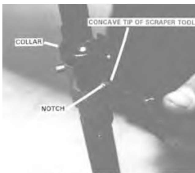
Step 1. Placement of the Scraper Tool.
