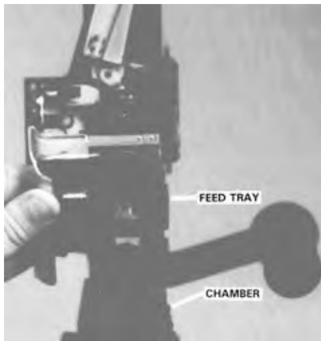
Figure 3-60. Inspecting the Chamber.
