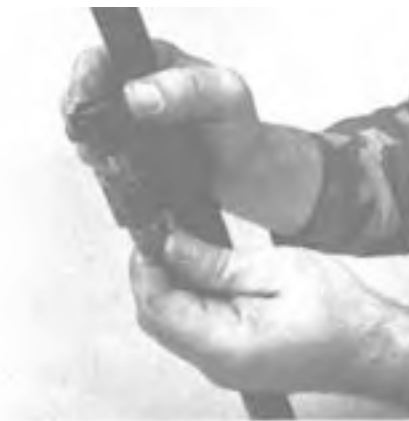
Step 2. Removing Collar From Gas Plug.
