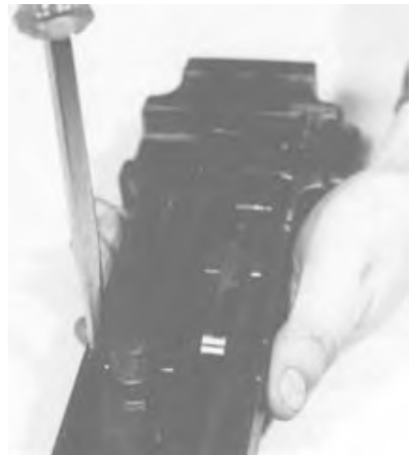
Figure 4-38. Removing the Belt Feed Lever.
