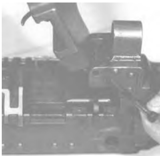
Figure 4-37. Removing the Cover Group.
