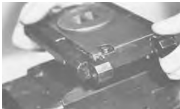
Figure 5-13. Rotation of Sear Housing Assembly.
