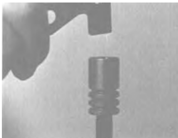
Figure 2-40. Cleaning the Hole in the Front of the Piston.
