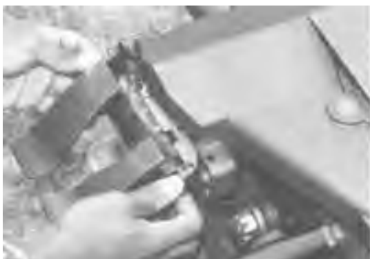
Figure 5-48. Attach Feed Throat to Feeder.
