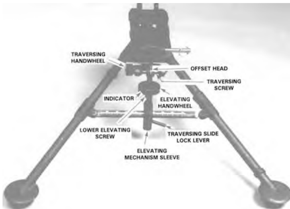
Figure 3-41. T&E Mechanism.
