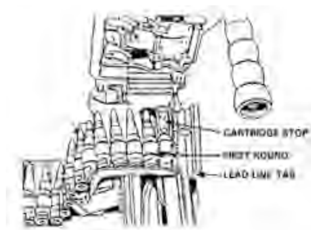
Figure 2-42. Cartridges in Metallic Belt.
