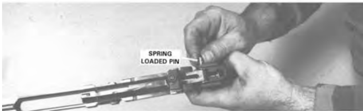
Step 2. Inserting the Spring Loaded Pin.
