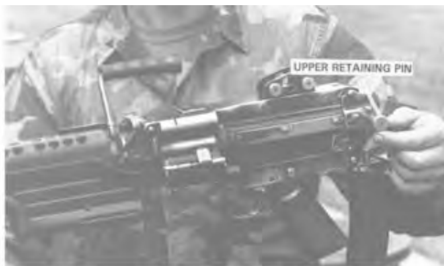
Step 1. Rotating the Buttstock Down.
