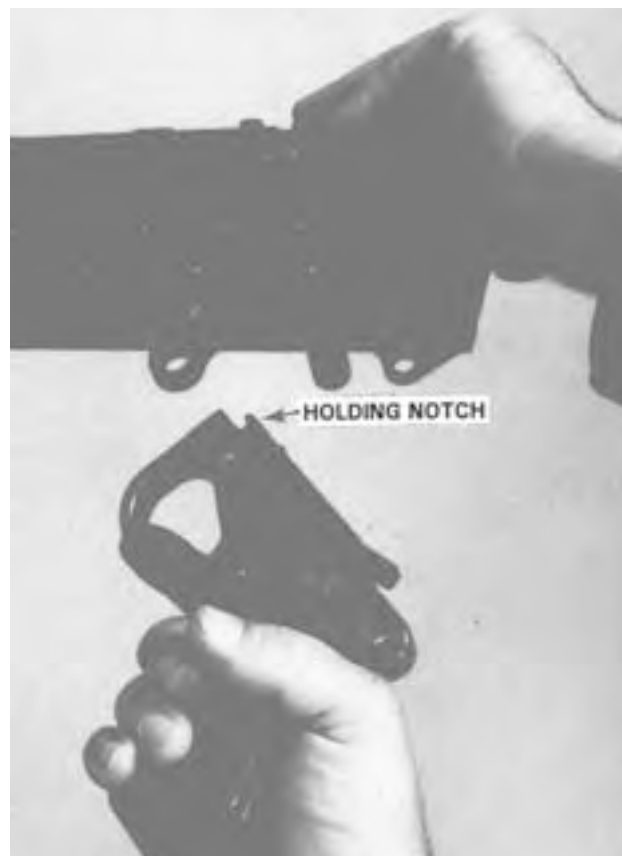
Figure 3-11. Replacing the Trigger Housing Group.
