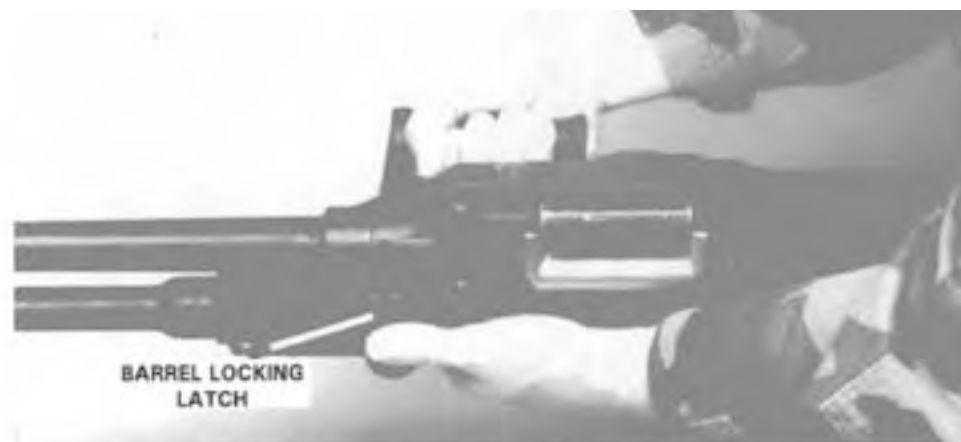
Step 1. Depressing the Barrel Locking Latch.
