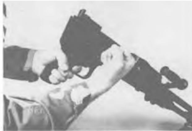
Step 1. Pulling the Cocking Handle to the Rear.
