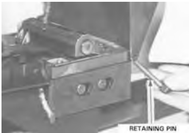
Figure 5-10. Removing the Feed Tray Cover Retaining Pin.
