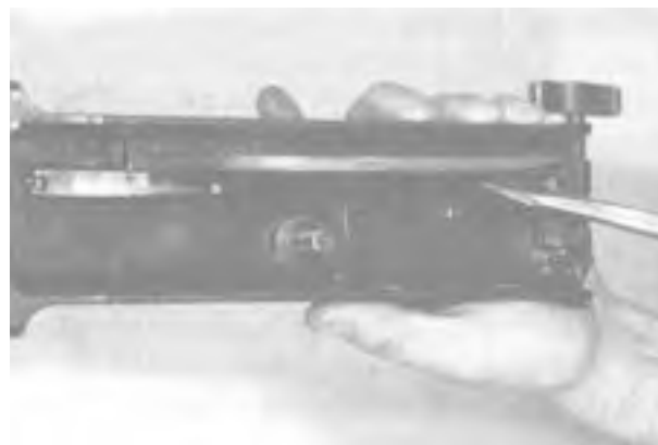
Figure 4-44. Removing the Cover Extractor Spring.
