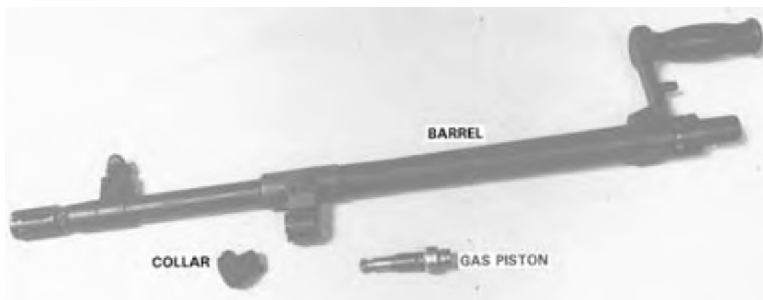
Figure 3-18. Barrel Group, Detailed Disassembly.
