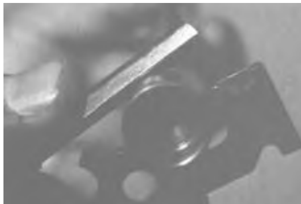
Figure 2-39. Cleaning the Grooves of the Piston.
