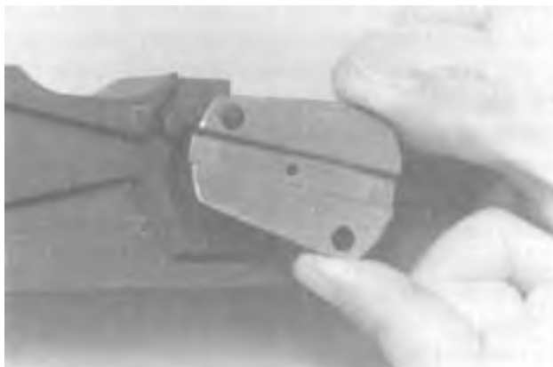
Figure 4-33. Replacing the Bolt Switch and Stud.
