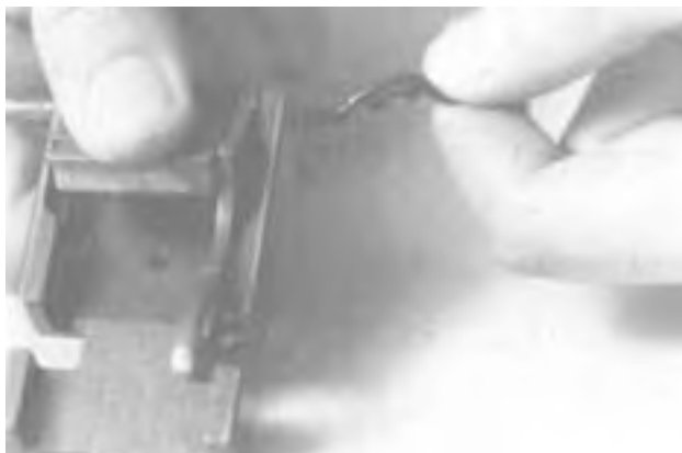
Figure 4-41. Drifting Out the Belt Feed Pawl Pin.
