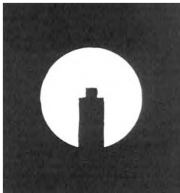
Figure 4-106. Correct Sight Picture.
