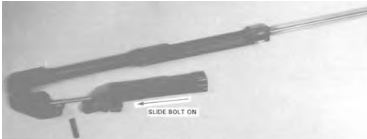
Step 1. Sliding the Bolt Over Firing Pin.
