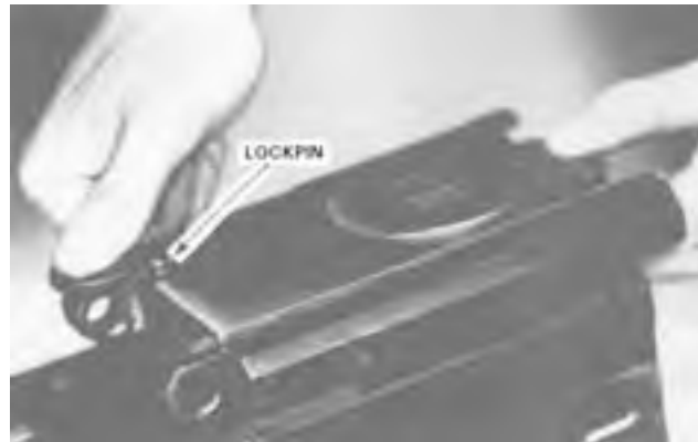
Figure 5-12. Lifting the Locking Pin.
