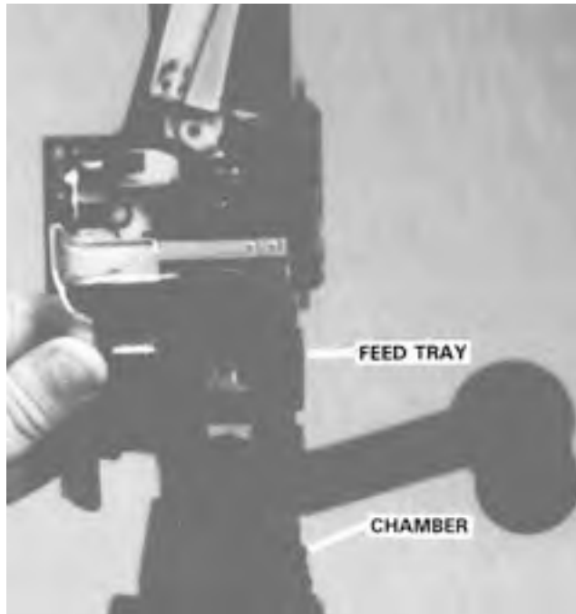
Figure 3-60. Inspecting the Chamber.
