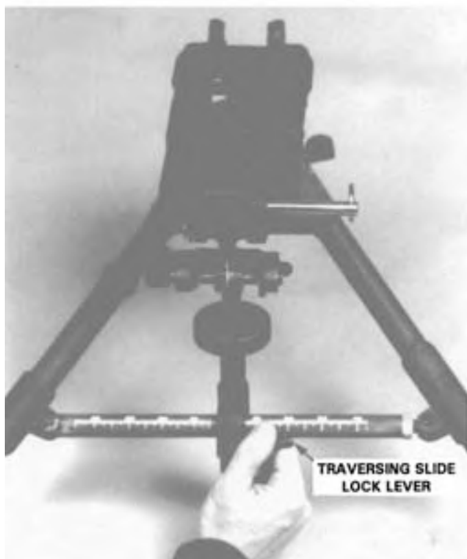
Figure 3-42. Attaching the Flex-mount to the Tripod—Continued.
