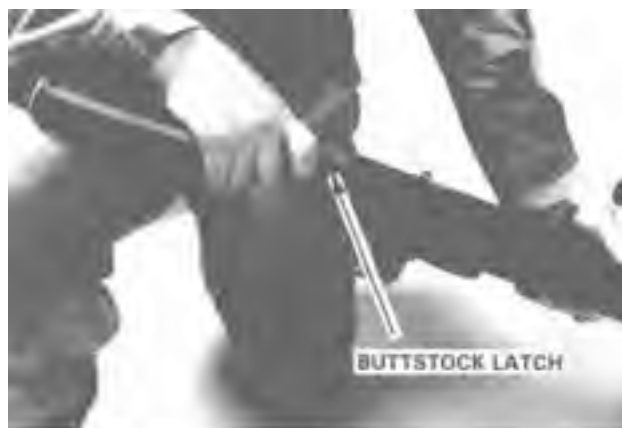
Step 1. Depressing the Buttstock Latch.
