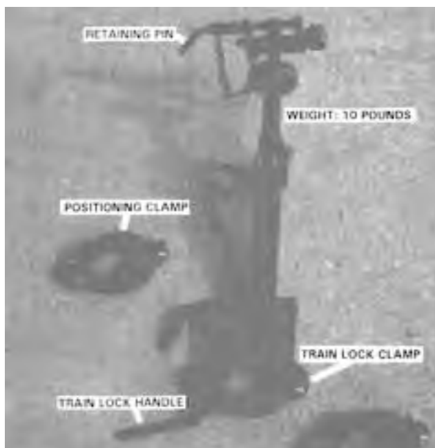
Figure 5-41. T&E Mechanism Mount Assembly.
