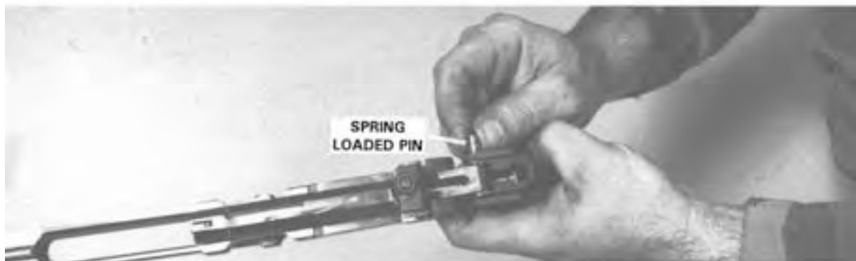
Step 2. Inserting the Spring Loaded Pin.
