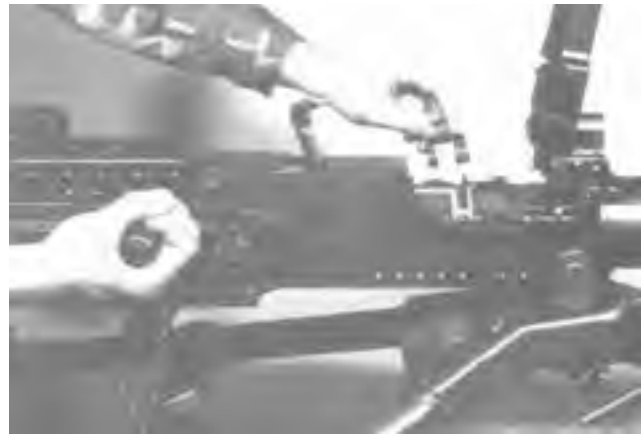
Figure 4-5. Aligning Barrel Locking Spring Lug With the 3/8-inch Hole.
