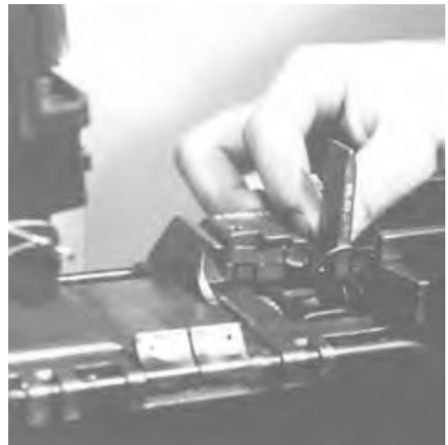
Figure 4-52. Inserting the Headspace Gage.
