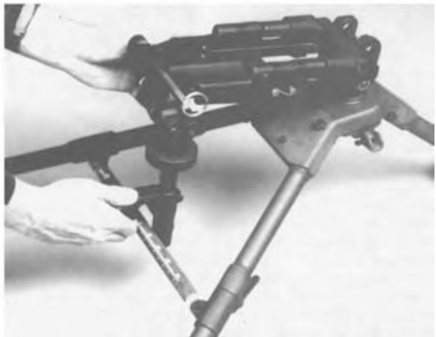
Figure 3-42. Attaching the Flex-mount to the Tripod.
