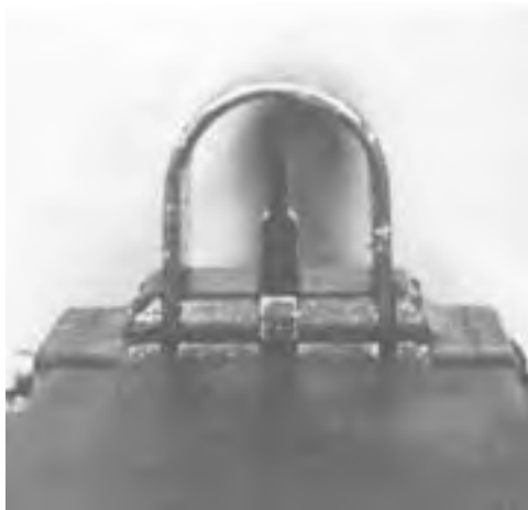
Figure 4-3. Front Sight, Cover, and Blade.
