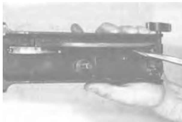
Figure 4-44. Removing the Cover Extractor Spring.
