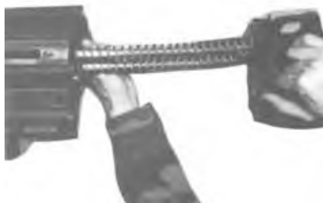
Figure 5-8. Removing the Bolt and Backplate Assembly.
