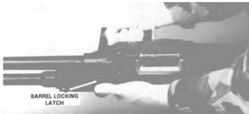
Step 1. Depressing the Barrel Locking Latch.
