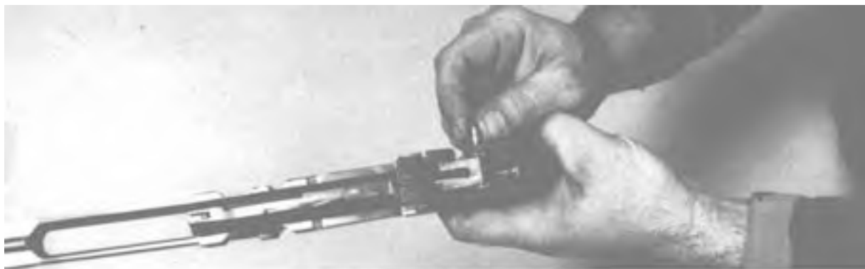
Step 1. Removing the Spring Loaded Pin.
