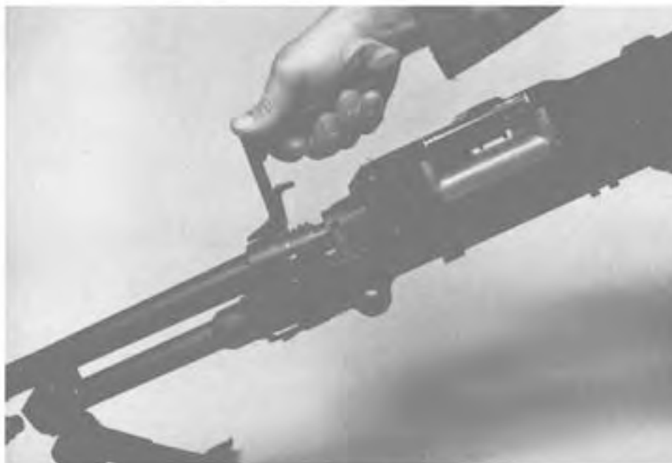
Step 2. Rotating Barrel Changing Handle Upright and Pulling Forward to Remove Barrel from Receiver.
