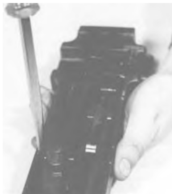
Figure 4-38. Removing the Belt Feed Lever.
