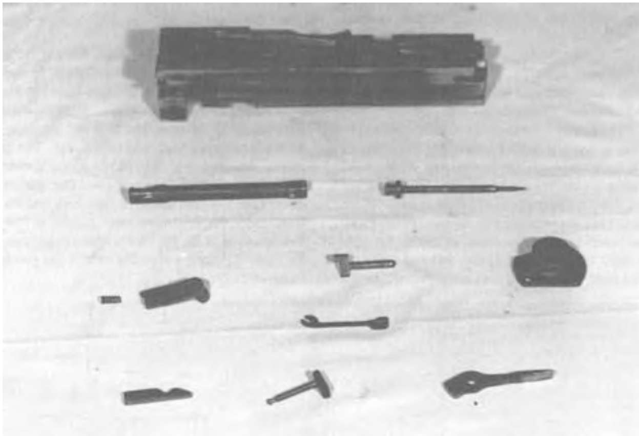
Figure 4-19. Bolt Group, Exploded View.
