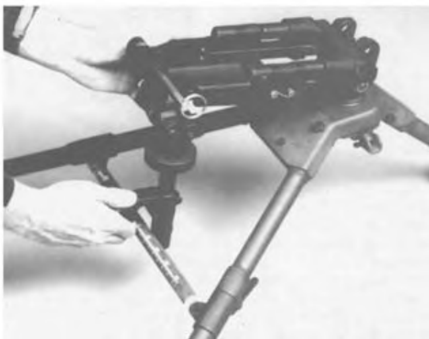
Figure 3-42. Attaching the Flex-mount to the Tripod.
