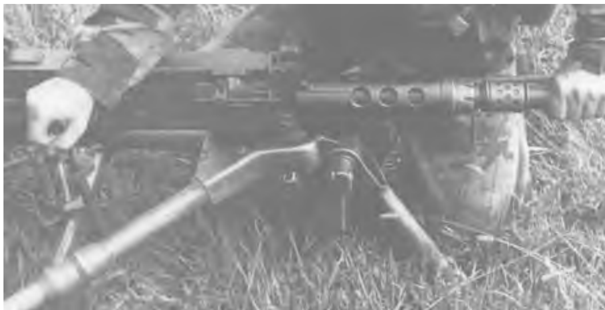
Figure 4-7. Removing the Barrel.
