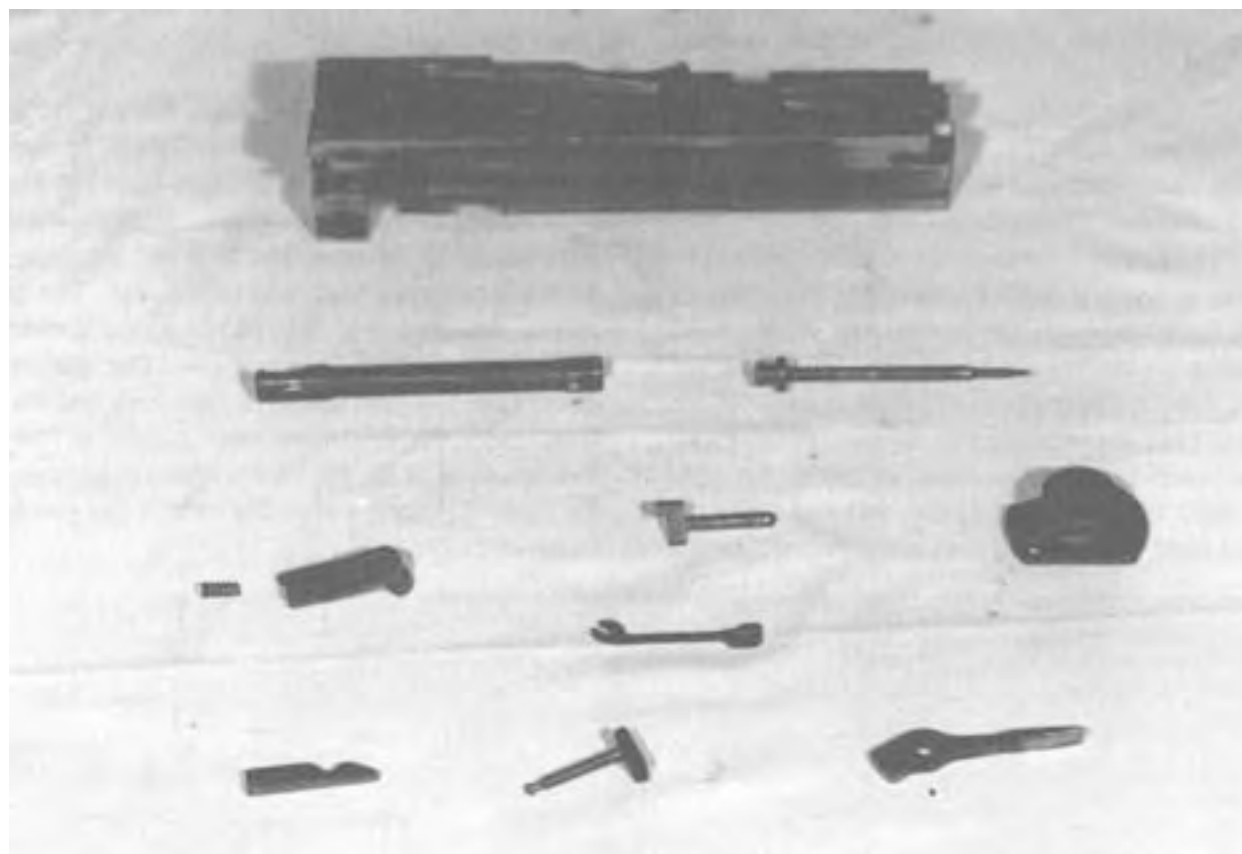
Figure 4-19. Bolt Group, Exploded View.
