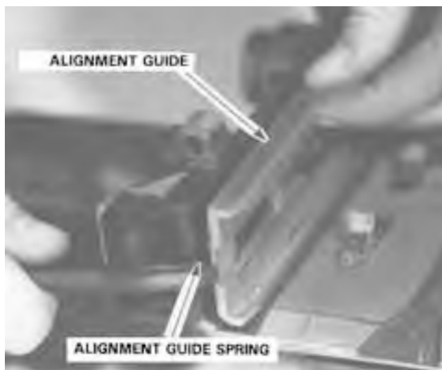
Figure 5-19. Removing the Alignment Guide Assembly.
