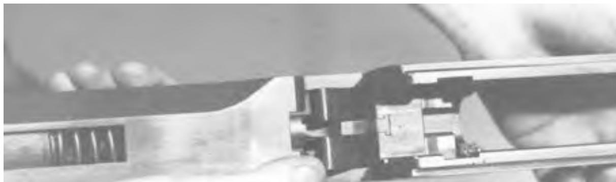
Figure 4-18. Joining the Barrel Extension Group and Barrel Buffer Group.
