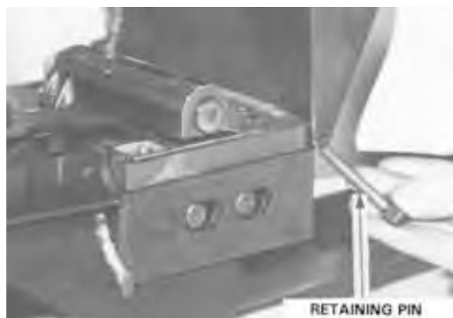
Figure 5-10. Removing the Feed Tray Cover Retaining Pin.
