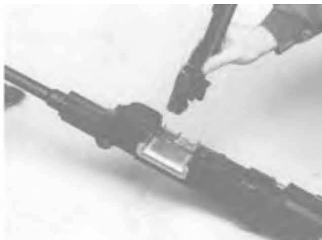
Step 2. Removing the Cover and Feed Tray.
