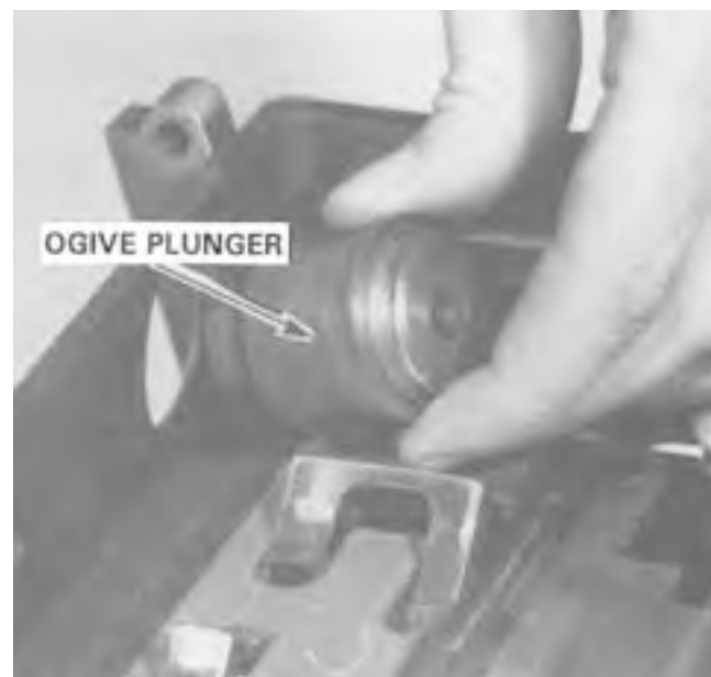
Figure 5-20. Removing the Ogive Plunger.
