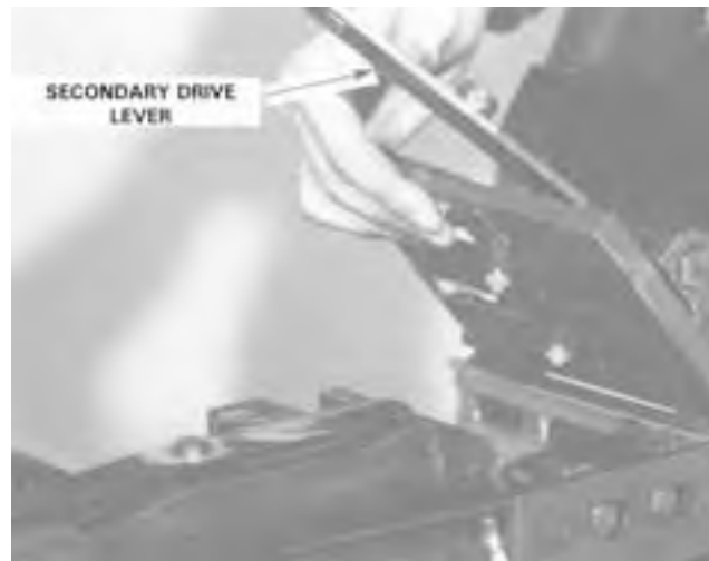
Figure 5-9. Removing the Secondary Drive Lever.
