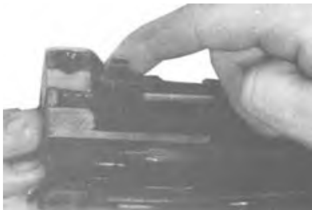
Figure 4-22. Removing the Cocking Lever and Cocking Lever Pin.
