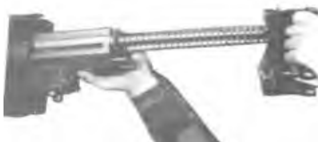
Figure 5-15. Depressing the Sear While Sliding the Bolt Assembly Forward.
