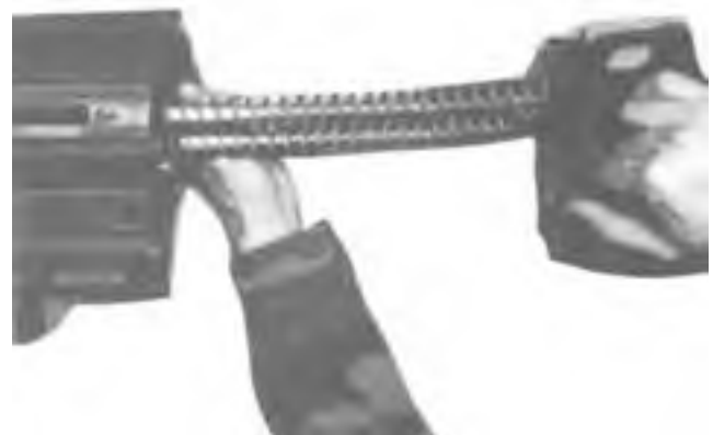
Figure 5-8. Removing the Bolt and Backplate Assembly.
