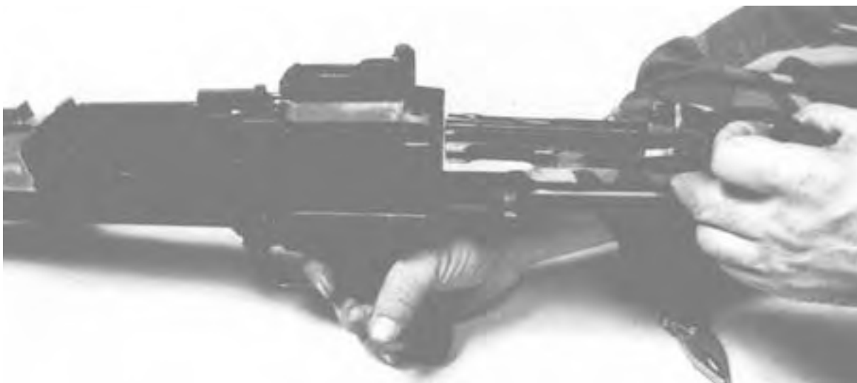
Figure 3-12. Replacing the Bolt and Operating Rod Assembly.
