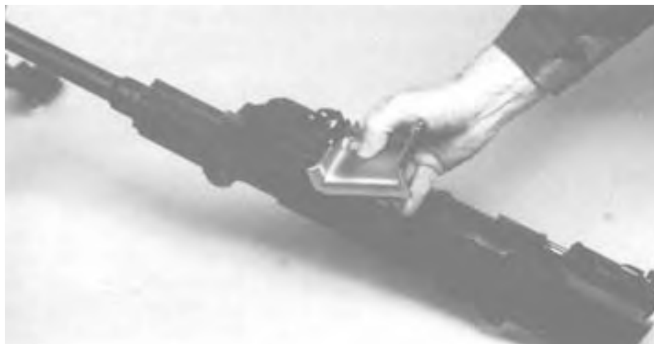
Figure 3-21. Aligning the Feed Tray Guides.
