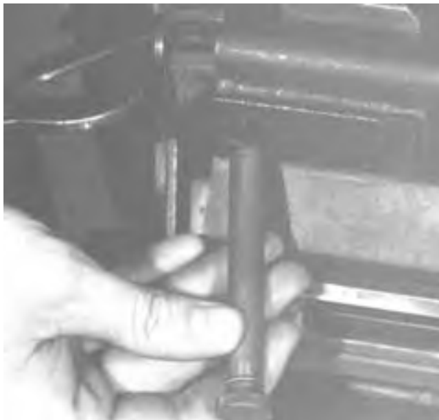
Figure 5-7. Removing the Bolt and Backplate Pin.
