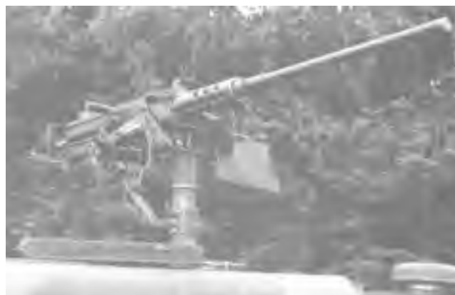
Figure 4-71. HMMWV Mount With MK64 MOD 5 Cradle.
