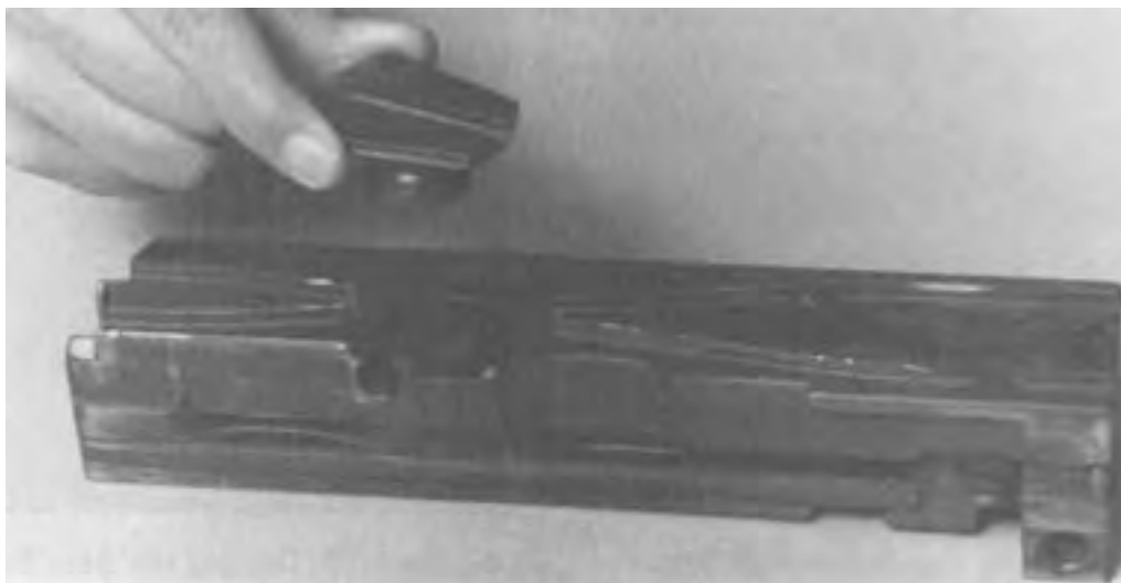
Figure 4-21. Removing the Bolt Switch and Bolt Switch Stud.
