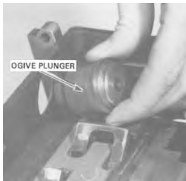
Figure 5-20. Removing the Ogive Plunger.
