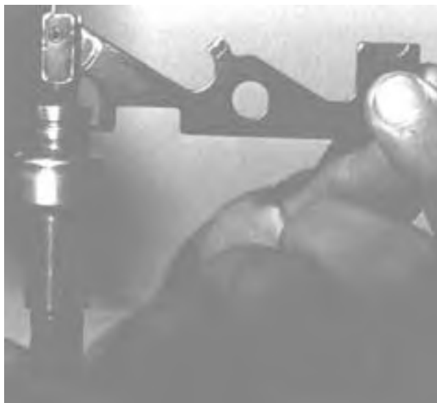
Figure 2-37. Cleaning the Grooves of the Body.
