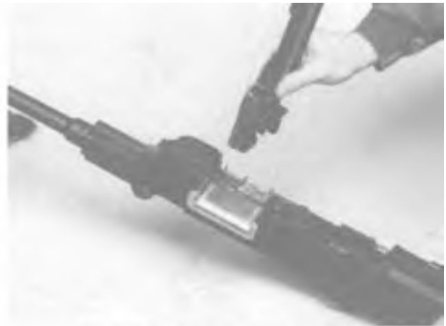
Step 2. Removing the Cover and Feed Tray.
