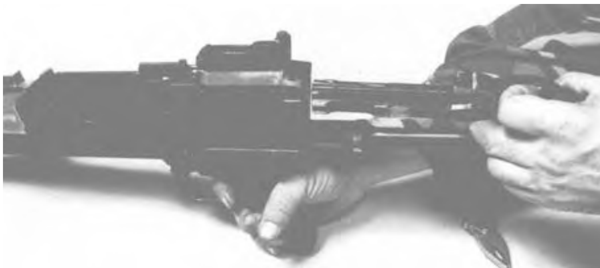
Figure 3-12. Replacing the Bolt and Operating Rod Assembly.
