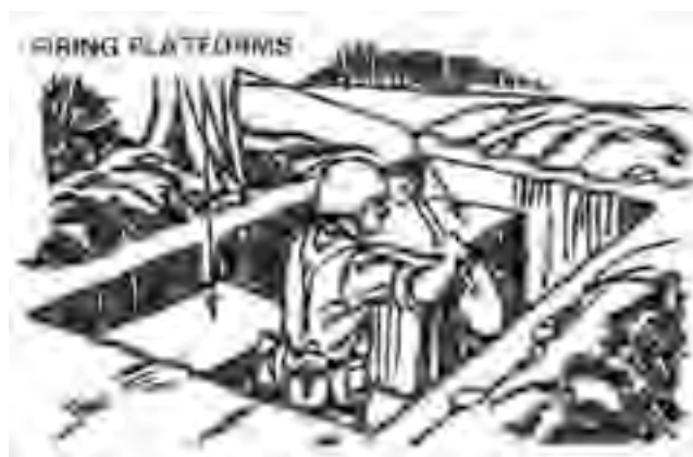
Figure 6-69. Digging T-Shaped Position.
