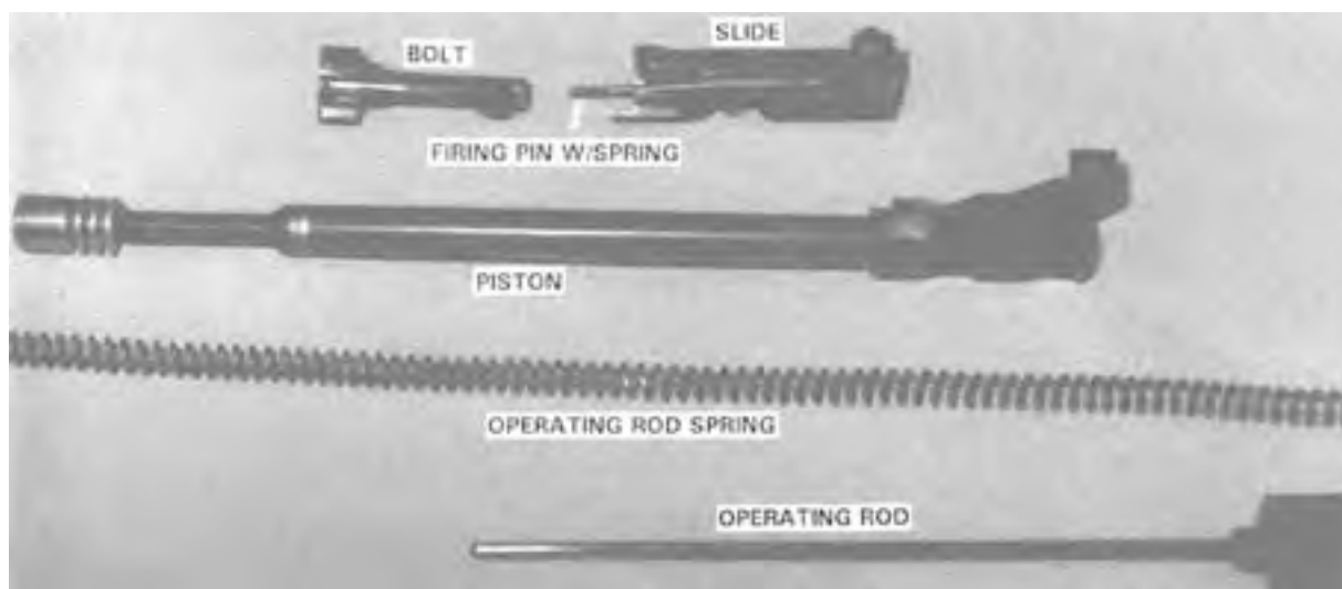
Figure 2-15. Operating Group, Detailed Disassembled.
