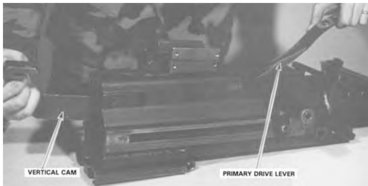
Figure 5-18. Removing the Primary Drive Lever and Vertical Cam.
