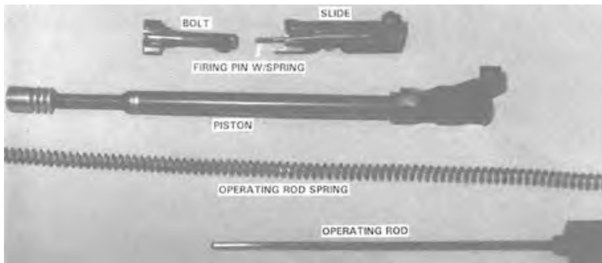
Figure 2-15. Operating Group, Detailed Disassembled.
