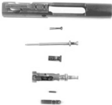
Figure 2-17. Bolt Carrier Disassembled.
