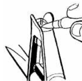
Figure 9-3. Front Sight Adjustment.
