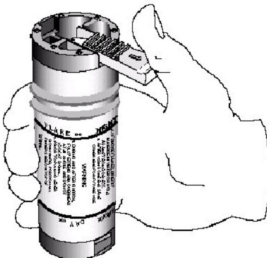
Figure 6-13 Operating the MK-124 MOD 0 Signal Flare
