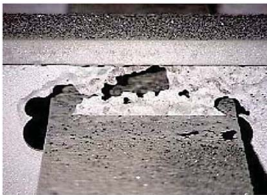
Figure 1-11. Examples of Concentration/Crevice Corrosion
