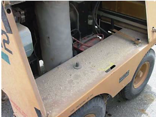
Figure 7-2. Sand/Dust Intrusion
