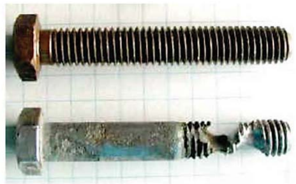
Figure 1-11. Examples of Concentration/Crevice Corrosion
