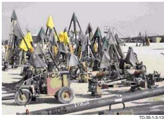
Figure 7-4. Locally Manufactured Permeable Covers
