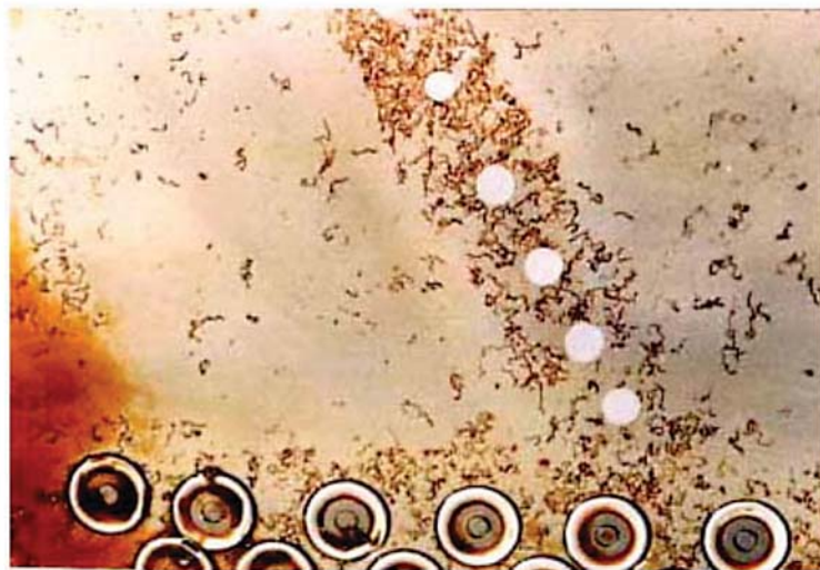
Figure 1-13. Example of Filiform Corrosion
