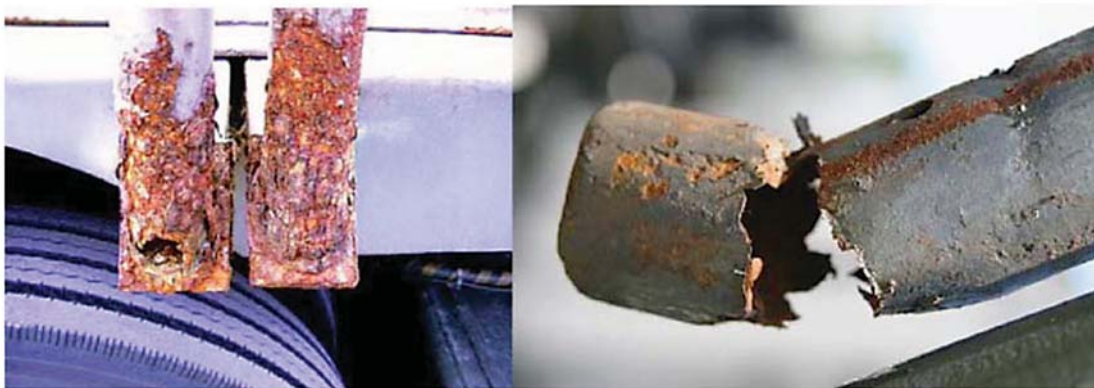
Figure 1-3. Corrosion Accelerated by Condensed Moisture
