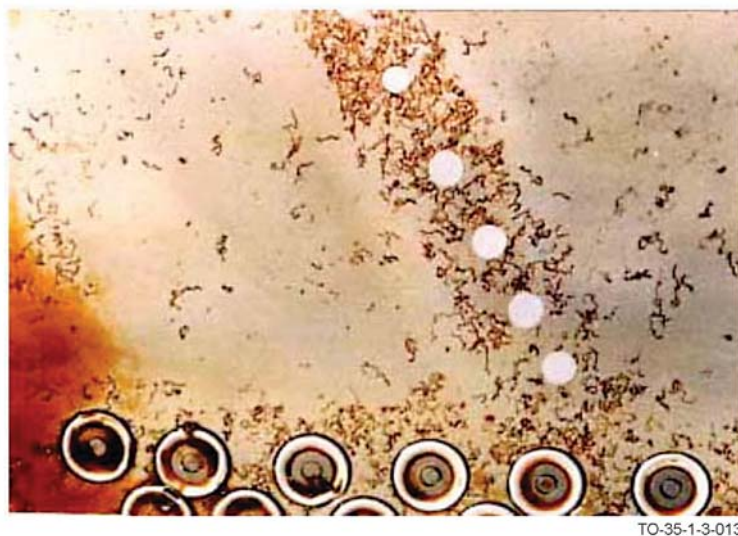
Figure 1-13. Example of Filiform Corrosion
