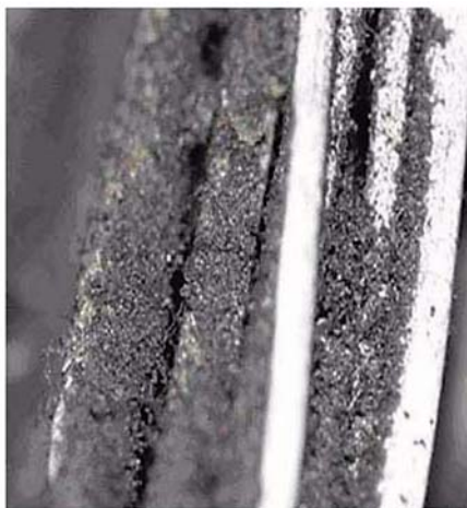
Figure 7-5. Wire Bundle Sand/Dust Accumulation
