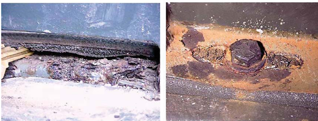
Figure 1-4. Open Cell Foam and Resulting Corrosion
