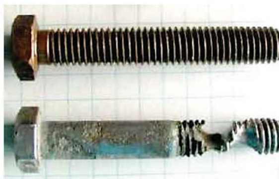
Figure 1-11. Examples of Concentration/Crevice Corrosion
