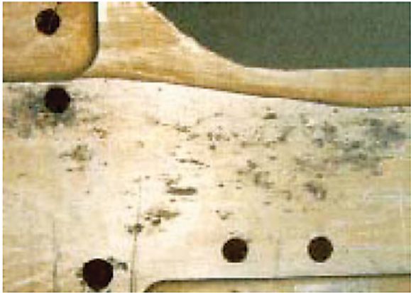
Figure 1-8. Example of Pitting Corrosion
