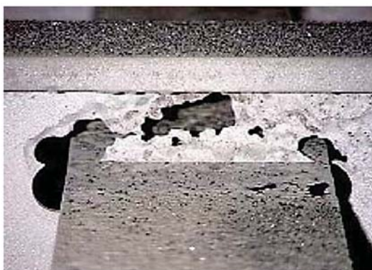
Figure 1-11. Examples of Concentration/Crevice Corrosion
