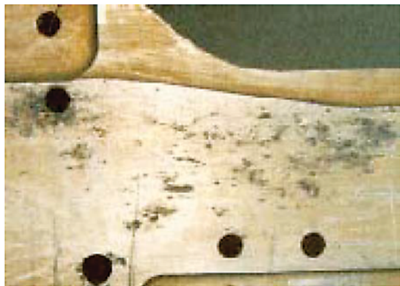
Figure 1-8. Example of Pitting Corrosion
