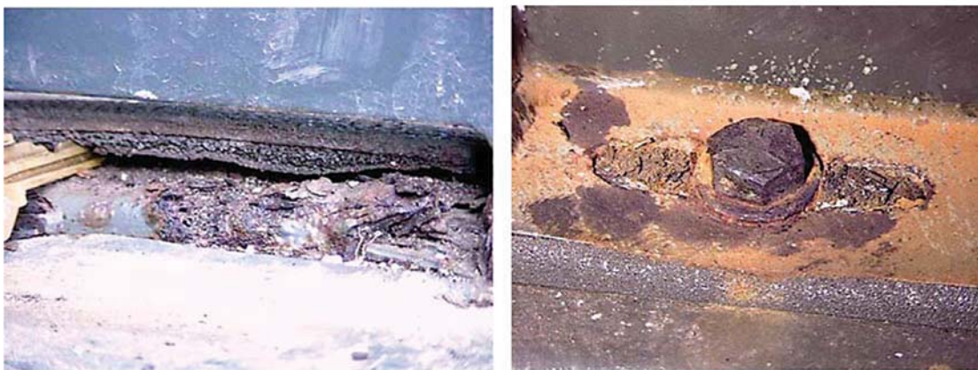
Figure 1-4. Open Cell Foam and Resulting Corrosion
