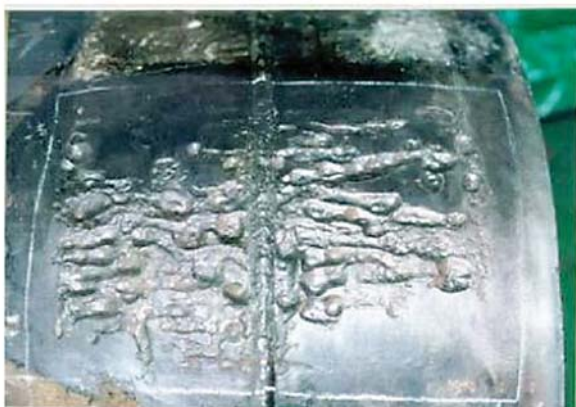
Figure 1-5. View of the Results of Microbial Induced Corrosion
