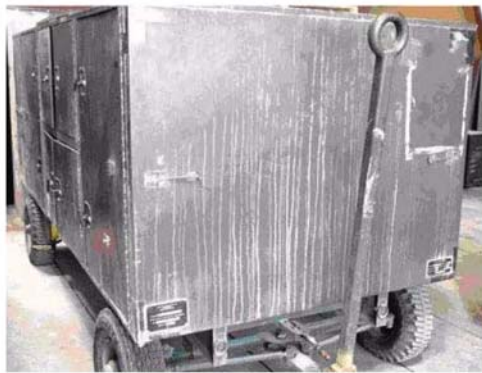
Figure 7-3. Residue from Salts Caused by Condensation
