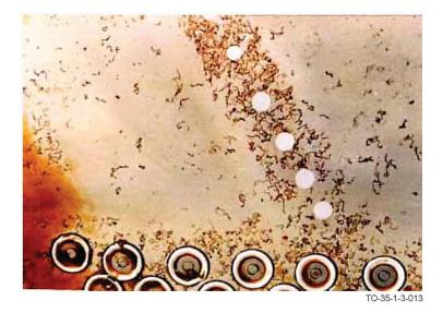
Figure 1-13. Example of Filiform Corrosion
