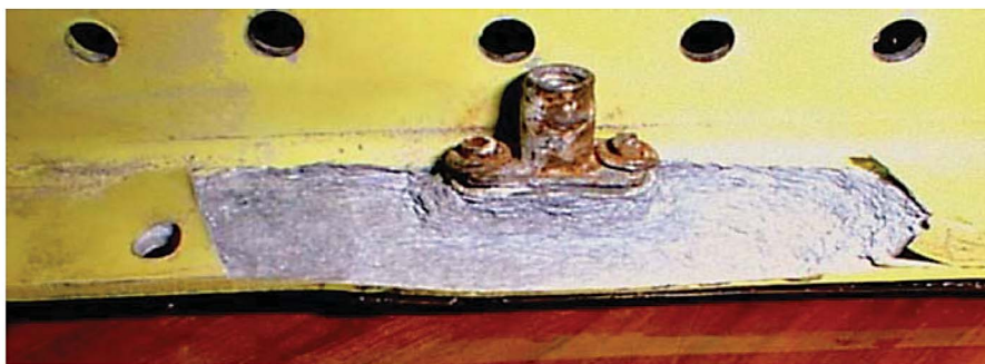
Figure 1-10. Example of Exfoliation Corrosion
