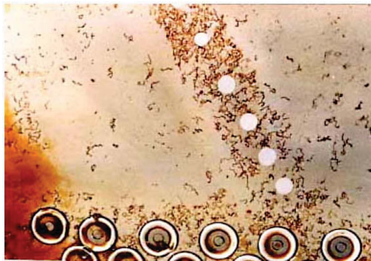
Figure 1-13. Example of Filiform Corrosion
