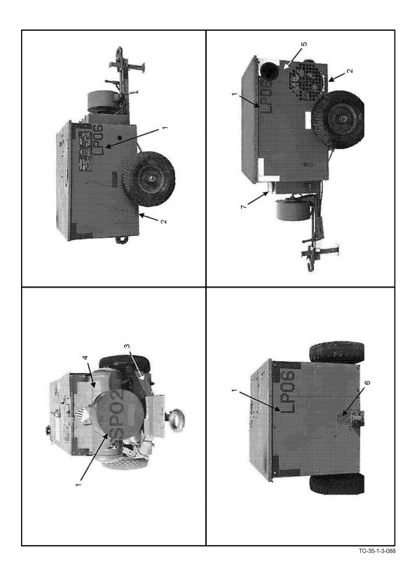
Figure 4-37. MC-2A Air Compressor (Sheet 1 of 2)
