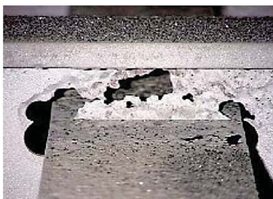
Figure 1-11. Examples of Concentration/Crevice Corrosion
