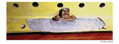
Figure 1-10. Example of Exfoliation Corrosion
