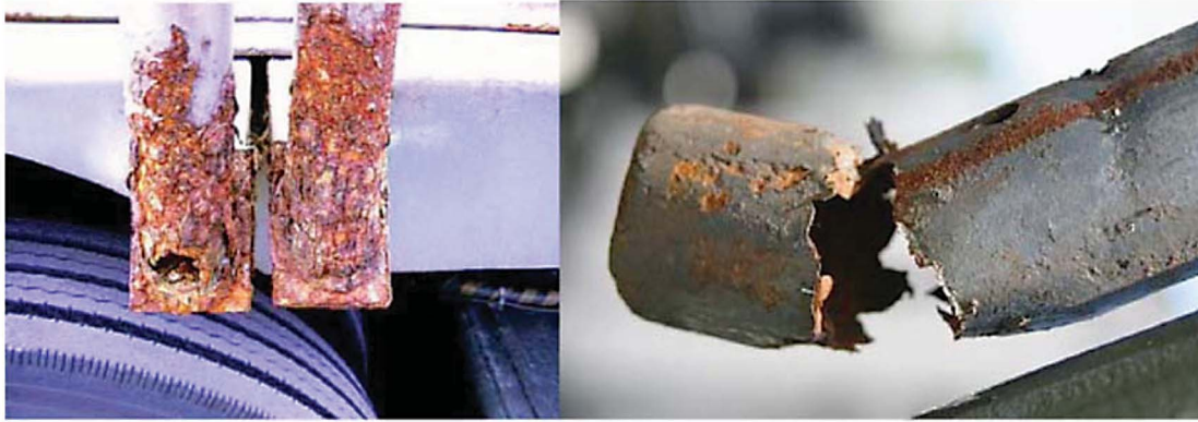
Figure 1-3. Corrosion Accelerated by Condensed Moisture
