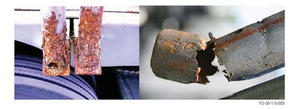
Figure 1-3. Corrosion Accelerated by Condensed Moisture
