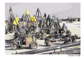
Figure 7-4. Locally Manufactured Permeable Covers
