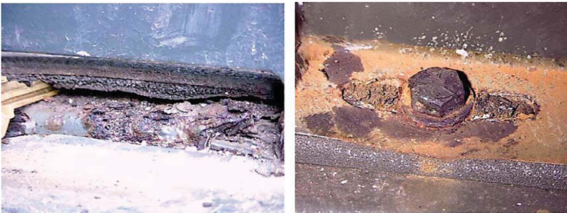
Figure 1-4. Open Cell Foam and Resulting Corrosion
