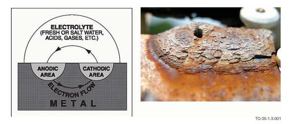
Figure 1-1. Diagram of a Simplified Corrosion Cell and an Example of Raised Corrosion Product
