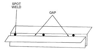
STRUCTURAL STEEL (ANGLE IRON) T GAPS/SEAMS TO-35-1-3-125
