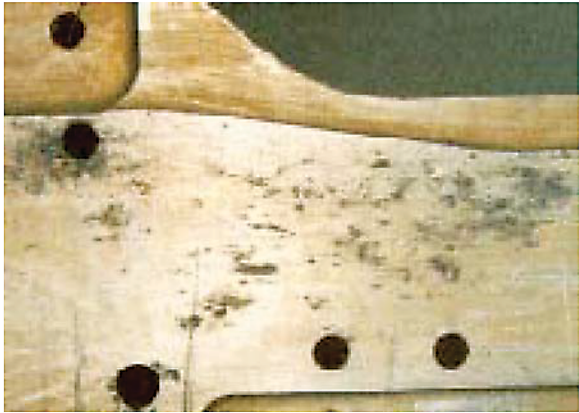
Figure 1-8. Example of Pitting Corrosion
