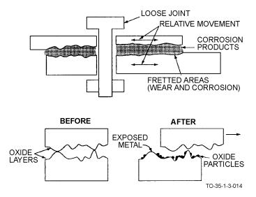
Figure 1-14. Illustration of a Fretting Corrosion Cell
