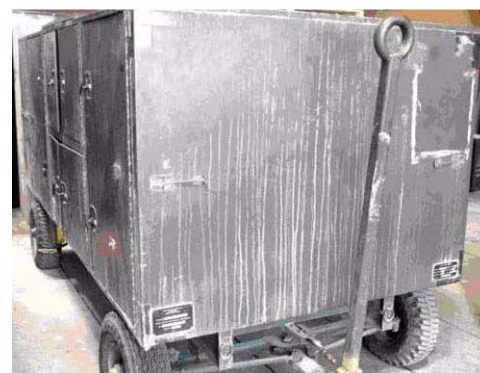
Figure 7-3. Residue from Salts Caused by Condensation
