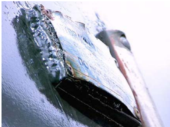
Figure 3-4. Corrosion Under Data Plate
