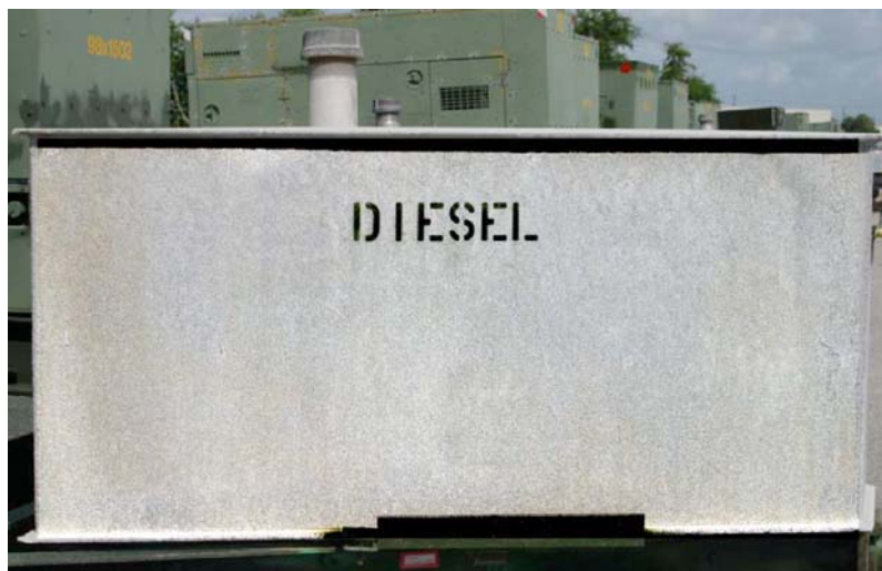
Figure 1-5. Example of Uniform Etch
