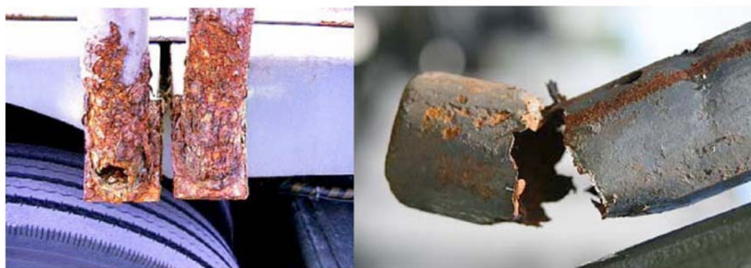
Figure 1-2. Corrosion Accelerated by Condensed Moisture
