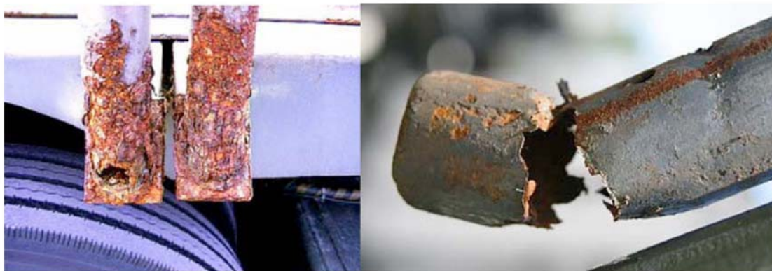
Figure 1-2. Corrosion Accelerated by Condensed Moisture
