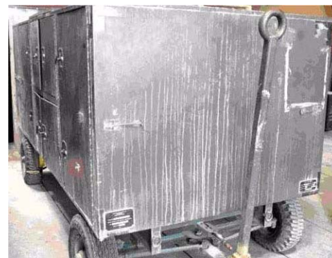
Figure 7-3. Residue from Salts Caused by Condensation
