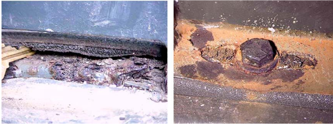
Figure 1-3. Open Cell Foam and Resulting Corrosion
