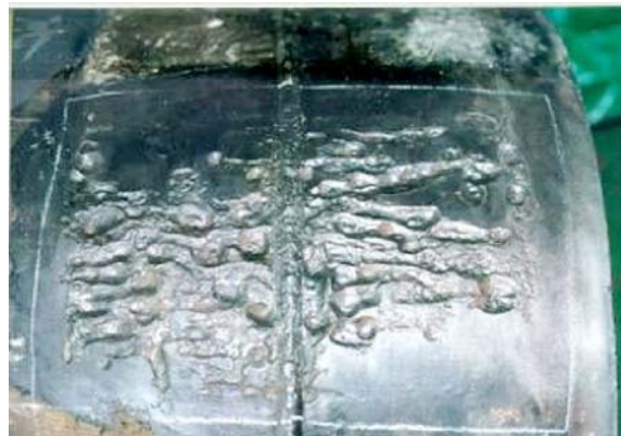
Figure 1-4. View of the Results of Microbial Induced Corrosion
