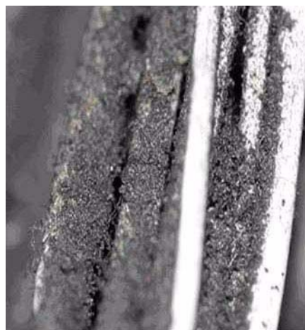
Figure 7-5. Wire Bundle Sand/Dust Accumulation
