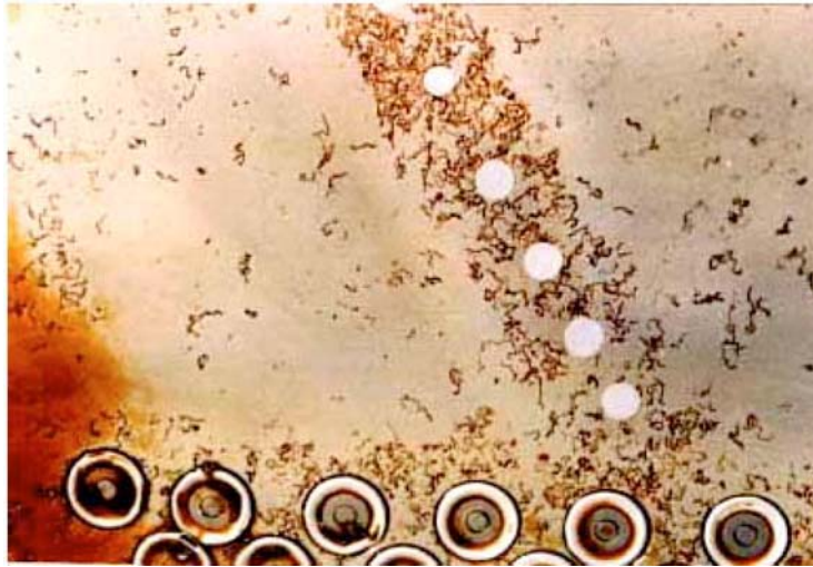
Figure 1-12. Example of Filiform Corrosion
