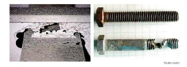
Figure 1-11. Examples of Concentration/Crevice Corrosion
