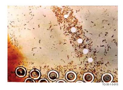
Figure 1-13. Example of Filiform Corrosion
