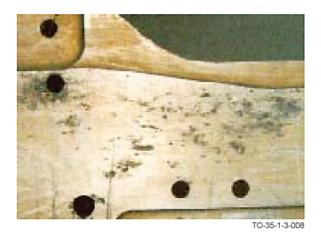
Figure 1-8. Example of Pitting Corrosion
