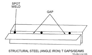
Figure 5-1. Angle Iron Sealant Application
