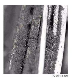
Figure 7-5. Wire Bundle Sand/Dust Accumulation
