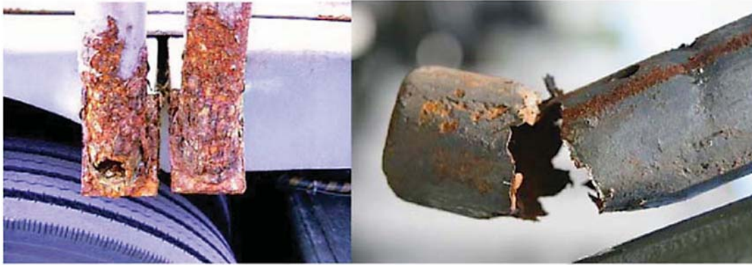
Figure 1-3. Corrosion Accelerated by Condensed Moisture
