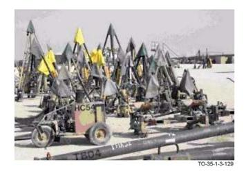
Figure 7-4. Locally Manufactured Permeable Covers
