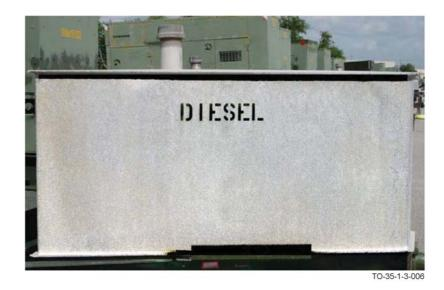
Figure 1-6. Example of Uniform Etch
