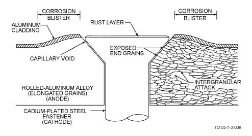
Figure 1-9. Illustration of an Intergranular Corrosion Cell
