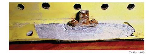
Figure 1-10. Example of Exfoliation Corrosion
