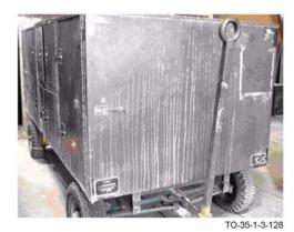
Figure 7-3. Residue from Salts Caused by Condensation
