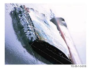
Figure 3-4. Corrosion Under Data Plate
