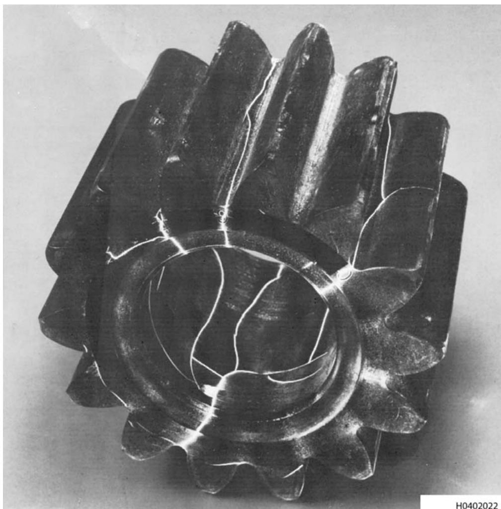
Figure 3-41. Typical Magnetic Particle Indications of Cracks
