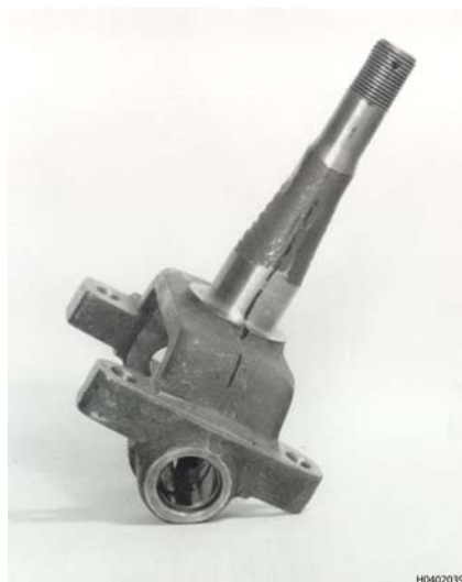
Figure 3-58. Magnetic Particle Indication of Flash Line Tear in a Partially Machined Automotive Spindle Forging
