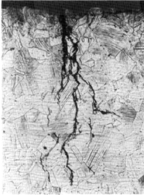
Figure 2-29. Micrograph of a Cross-Section Through a Stress-Corrosion Crack
