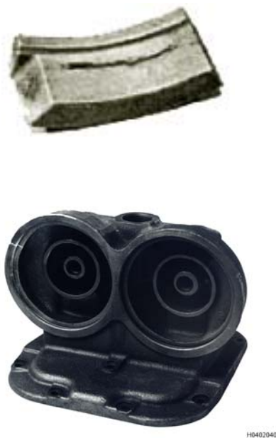
Figure 3-59. Magnetic Particle Indications of Defects in Castings
