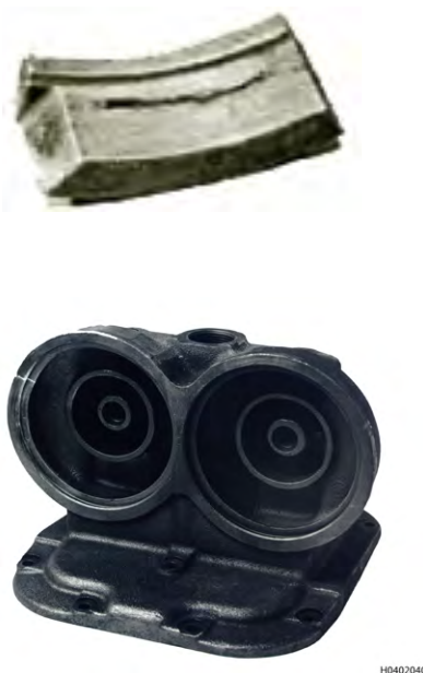
Figure 3-59. Magnetic Particle Indications of Defects in Castings
