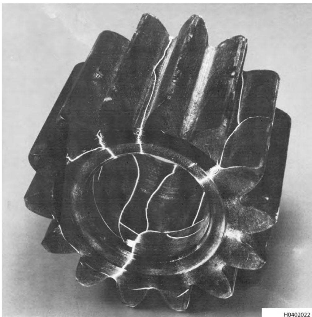
Figure 3-41. Typical Magnetic Particle Indications of Cracks
