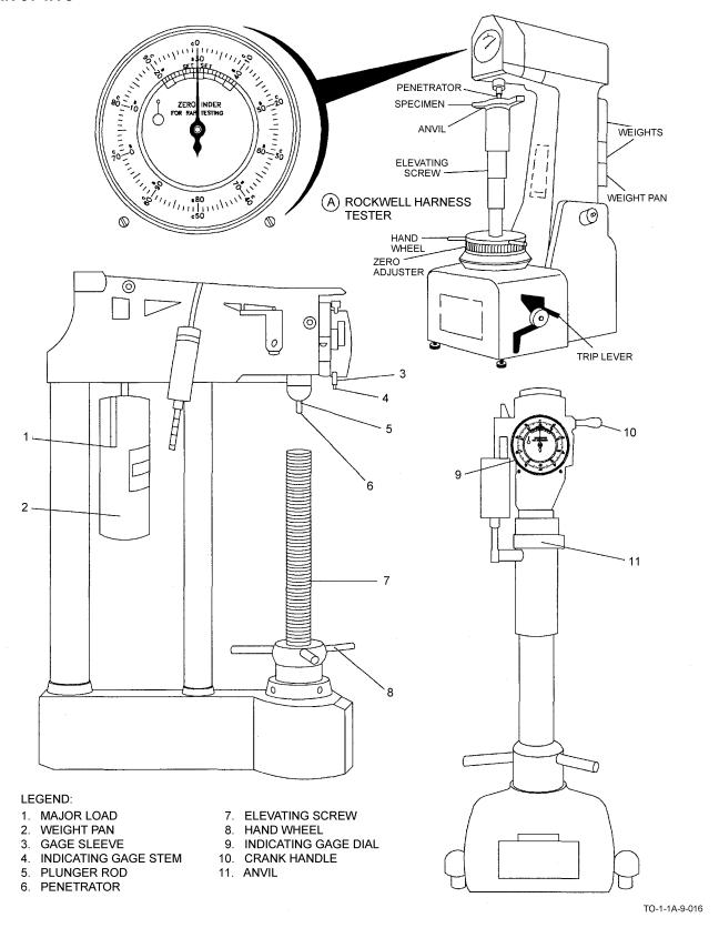
Figure 8-2. Rockwell Hardness Tester
