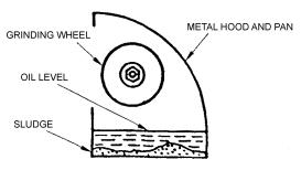
C TYPE OF DUST COLLECTOR FOR SMALL WHEELS USED ONLY INTERMITTENTLY AND WHEN SMALL AMOUNTS OF METAL ARE REMOVED.
