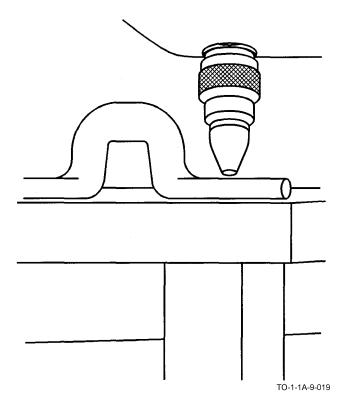
Figure 8-5. Standard Pyramid Diamond Indentor
