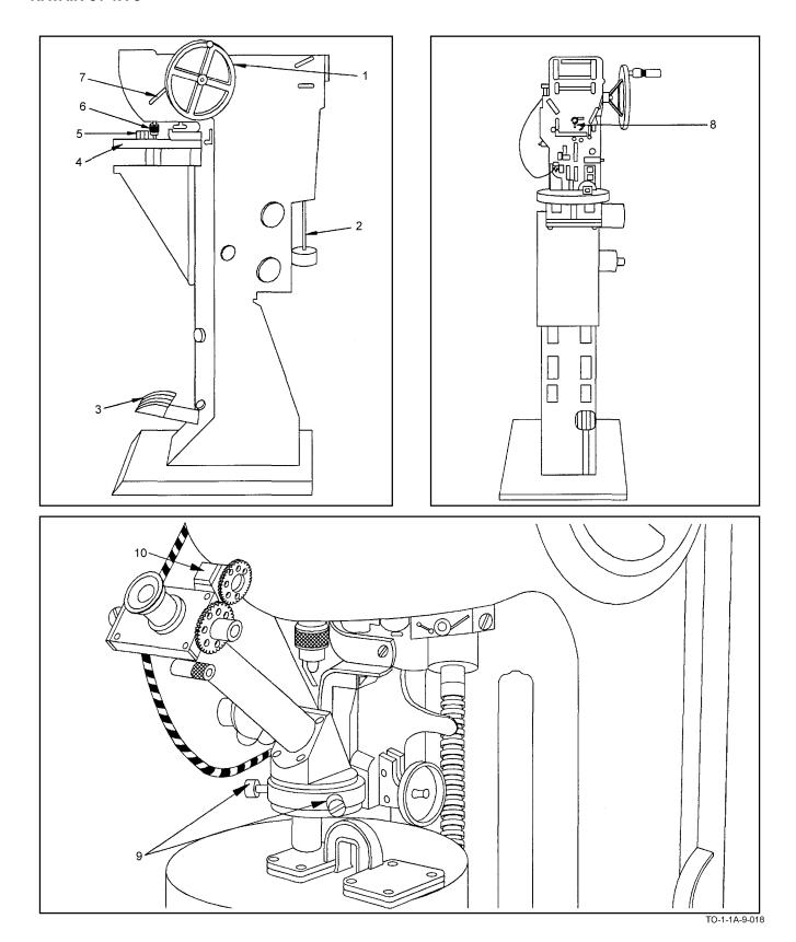
Figure 8-4. Vickers Pyramid Hardness Tester
