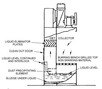
$\boldsymbol{\mathsf{B}}$  BENCH TYPE DUST COLLECTOR FOR USE WITH PORTABLE GRINDING OR POLISHING TOOLS.
